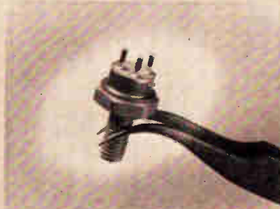
NPN silicon annular amplifier transistor (2N3818) provides 18 watts output power @ 100 mc using 25 volt source.
