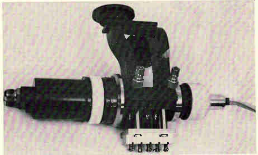
Klystron amplifier offers wide bandwidth, high gain and efficiency in a small package. The tube is 16.3 inches long and weighs only 22 pounds.
