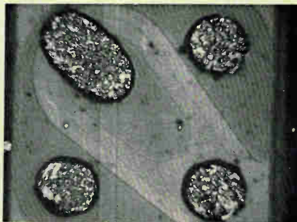
Bump-contacted chip. In this one, npn and pnp transistors share contacts 1 and 3. Photo shows top of chip. Large bump orients chip.
