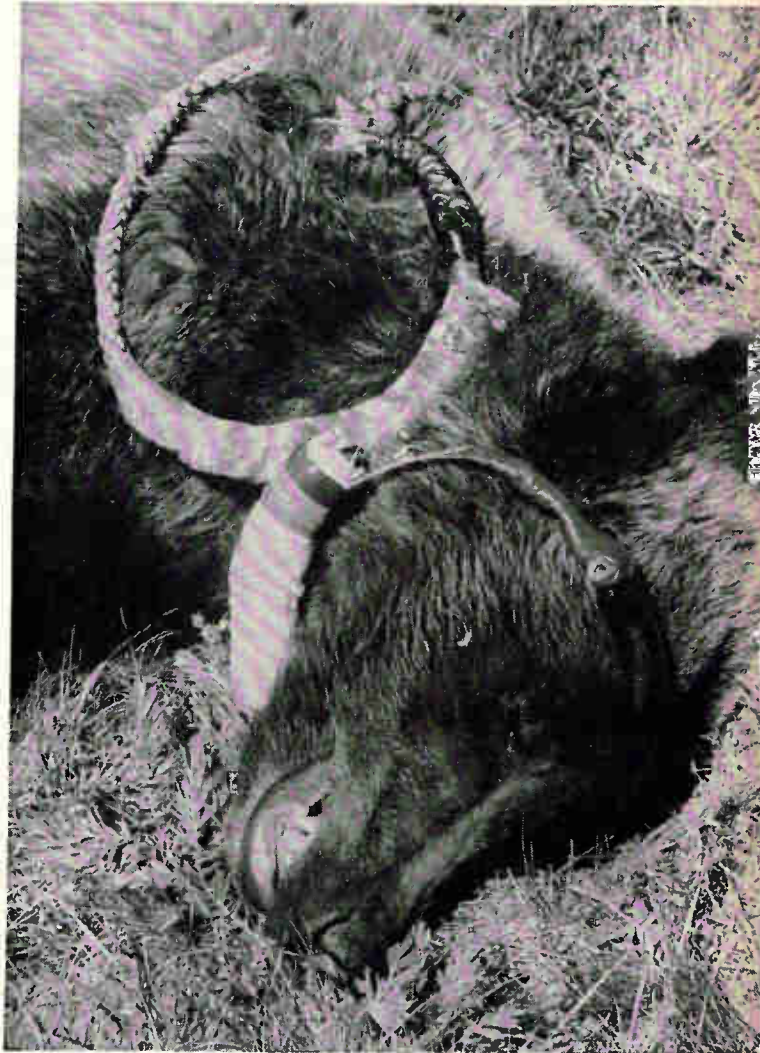
Transmitter in grizzly bear's collar is powered by seven mercury cells. It operates at 32.02 megacycles and has a range of 4 miles. It was designed by Frank and John Craighead, two physicians working with the Montana Cooperative Research Unit in Yellowstone National Park.
