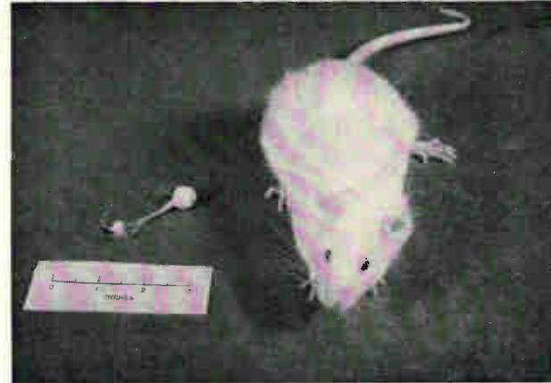
Biotelemetry transmitting package on the left is implanted beneath skin of a rat from the base of the skull to the tail. The unit, designed by Wen Ko of Case Institute, senses and transmits electrocardiograms more than 50 feet.
