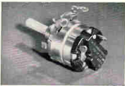
OCB breaker switch attached to volume control.
