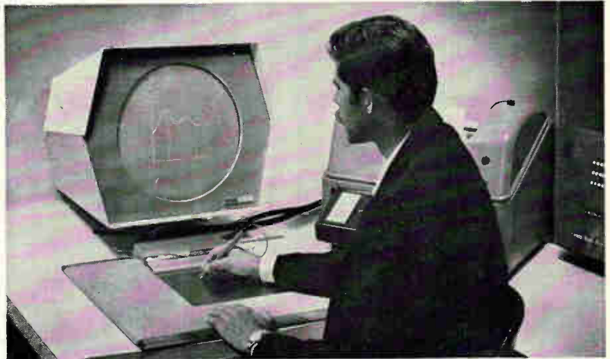
Data is "drawn" directly into computer with a stylus. The Grafacon 1010 translates the information, corrects it and adds to it—all in real time.
