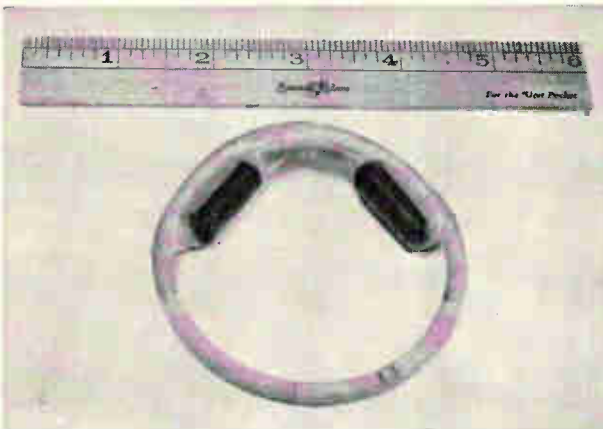
Low-power temperature-sensitive radio transmitter and its associated battery are inserted into the rim of an arching domeless diaphragm. Designed by Dr. Alvin Singer of American Electronic Laboratories, Inc., it continuously transmits vaginal temperatures for up to six months.
