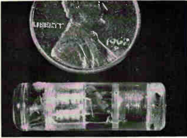
Intragastric pill, designed by R. B. Barrueto of the Boeing Co., is half the size of its predecessors, with a useful life at least 20 times greater. Acting as a pulse-position-modulation telemeter, it has a power output of 10-microwatts and a range of 75 feet. It can be used to monitor temperature, pressure or acceleration and pH (concentration of hydrogen ions in the blood).
