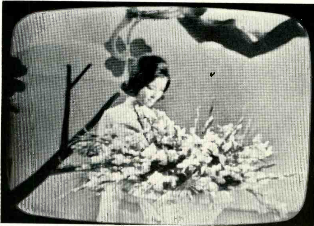
Scene photographed from the Yaou receiver shows how horizontal scanning across vertical phosphor stripes produces net-like appearance; hence the name, Colornet.
