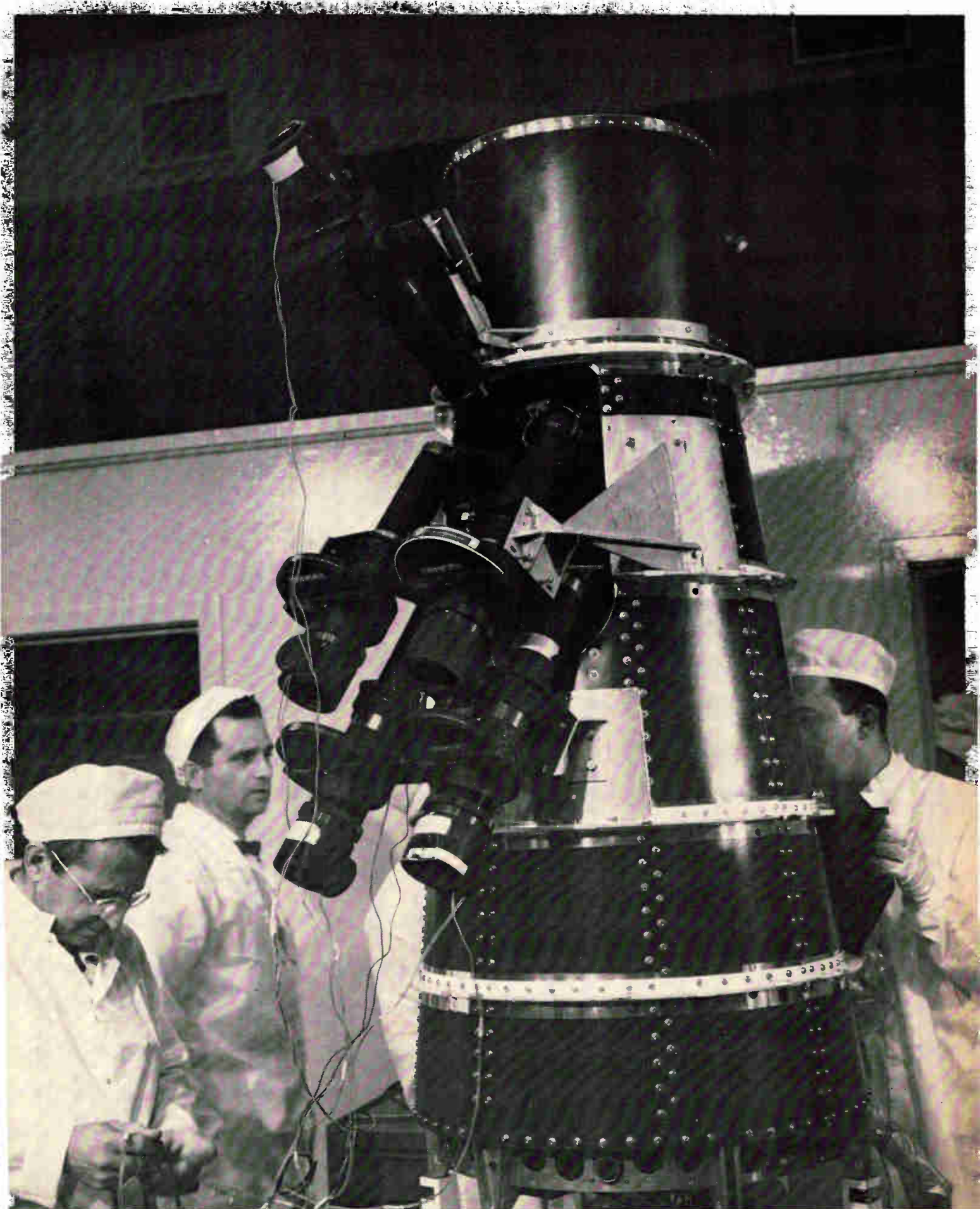
The 6 tv cameras used in the Ranger 9 spacecraft are checked out by engineers. Two wide-angle and four narrow-angle cameras were used.
