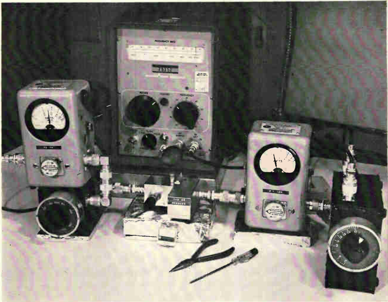
Test arrangement for 1-to-2-Gc doubler includes a wattmeter, at left, indicating the input power of 12 watts; a power oscillator set at 1 Gc; and another wattmeter, at right, showing the power output level of 7 watts at 2 Gc.
