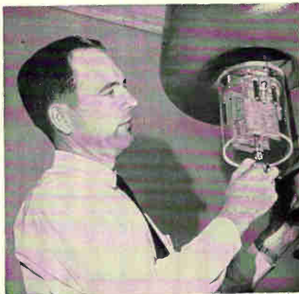
Plugging coder electronics into the head of a Traser system prior to prototype testing. Heavy magnetic shielding surrounds encoder unit to assure that passage of line current and resulting magnetic fields do not affect coder output accuracy appreciably.
