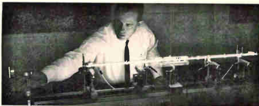
Frequency-modulated laser developed by Sylvania achieves a single-frequency output that retains the energy of all the modes of the original laser.
