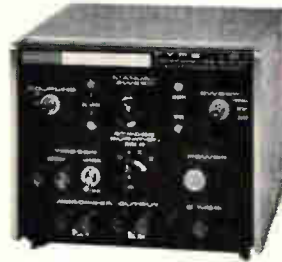
Type 101 Waveform Translator, converts high speed repetitive waveforms on an oscilloscope to accurately inked graphs with an x-y recorder, $675.
