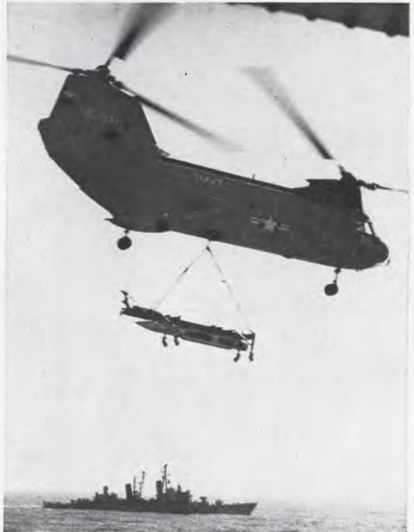
Navy's new utility helicopter is demonstrated in missile transfer exercises. The tandem rotor aircraft, built by the Boeing Co., Vertol division, can take off and land on water. Its hull is watertight.
