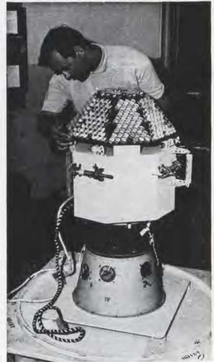
Explorer 22 has mirrors which reflect laser beams
