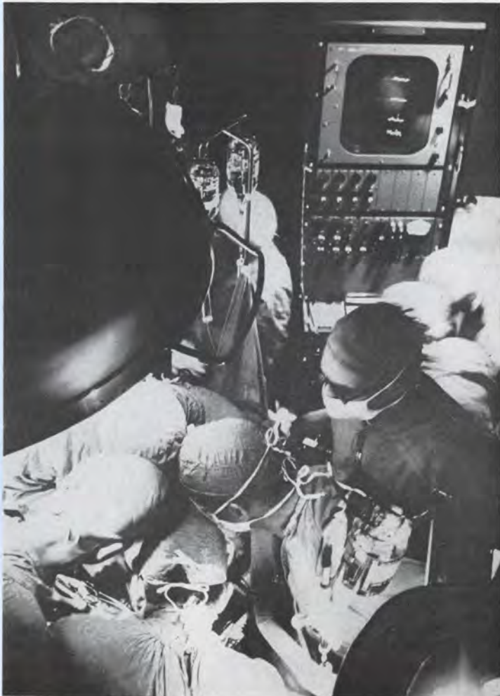
Electronic system in operating room measures depth of anesthetic and critical physiological reactions. The system, at upper right, is built by the Hewlett-Packard Co.
