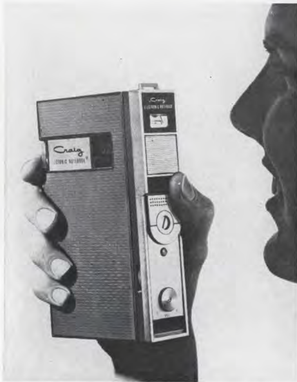
Tape recorder , built by Craig-Panorama, an "electronic notebook." It uses a half-hour tape pack and rechargeable nickel-cadmium batteries. Microphone is built in. Market for miniature tape recorders is considered strong.
