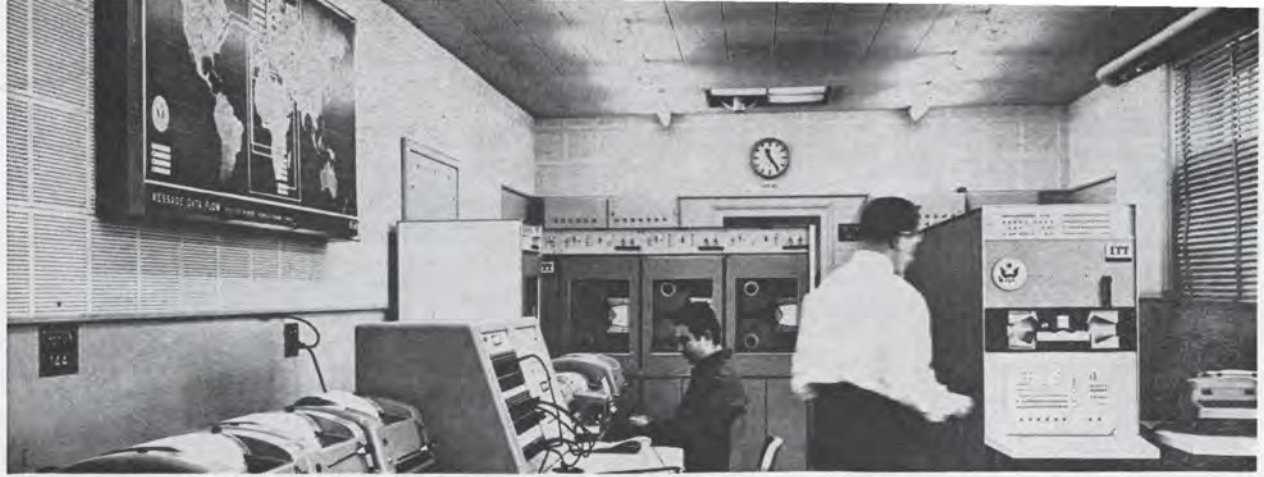
Nerve center for the State Department's communications operations in Europe is this Paris facility that switches and processes digital information. Developed by International Telephone and Telegraph Corp., the system accepts information from high-speed computers and slow-speed teleprinters, and stores low-priority messages for later transmission.
