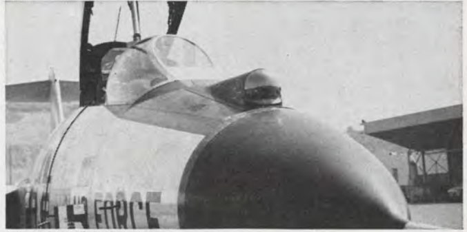
Interceptor IR installation
