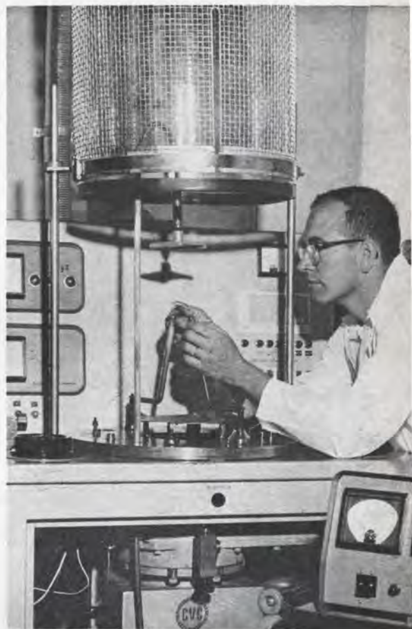
Donald M. Mattox converted a vacuum evaporator into an ion plater by putting insulated electrodes in the bell jar.
