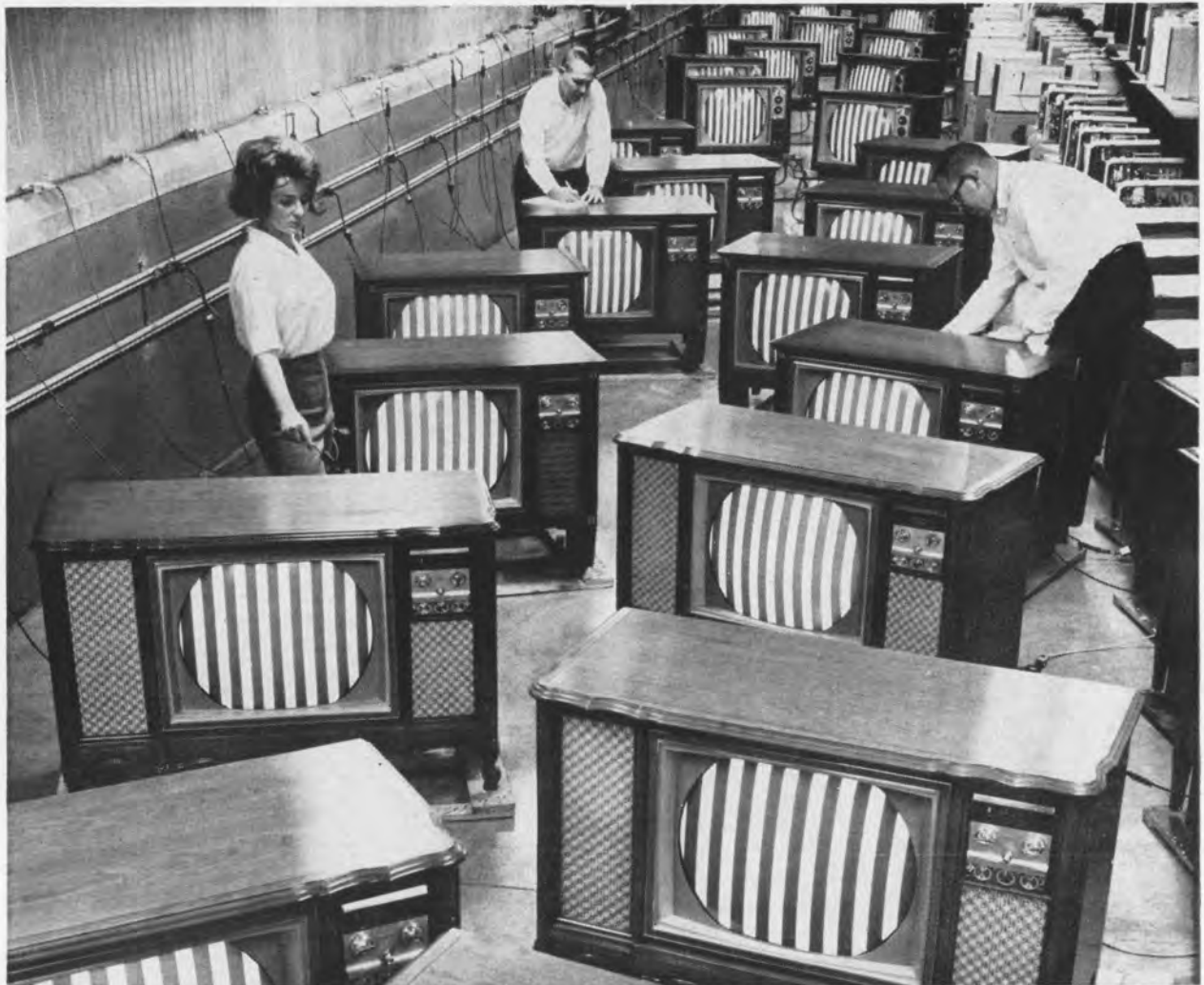
Color-tv receivers in Bloomington, Ind., tested at RCA Life-Test Labs. Many receivers are selected at random from this group for test and evaluation. Two million color-tv sets are expected to be sold in 1965.
