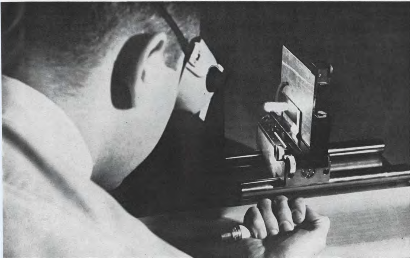
Laser welder system , developed by Union Carbide Corp., has a ruby-operated laser-head that produces a pulse output focused on the workpiece by an optical system. Laser welders are expected to be one of the most practical applications of high-energy coherent light.
