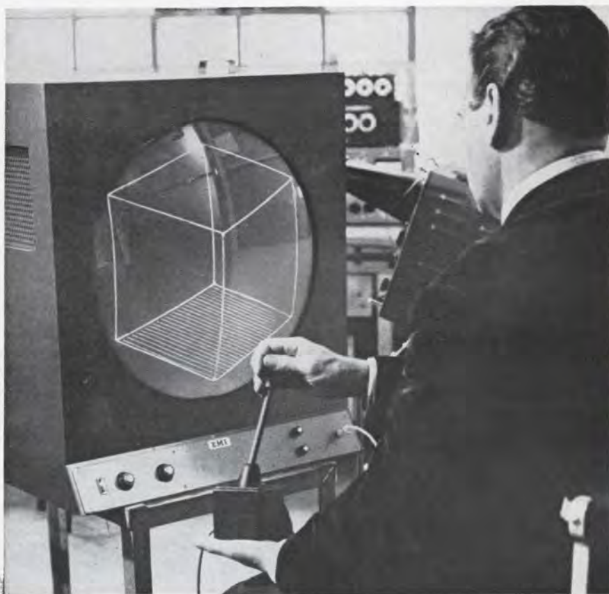
3-D radar picture is an image of a transparent cube representing airspace being controlled for air traffic. Within the cube, aircraft appear as luminous spots.
