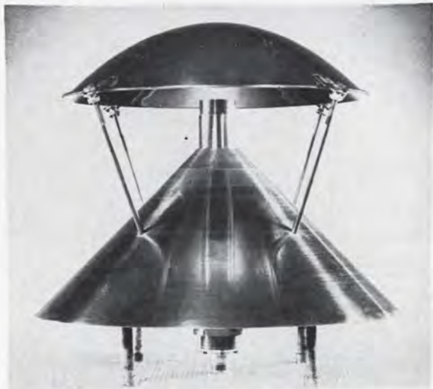
Microwave beacon antenna consists of a circular waveguide that illuminates a paraboloidal reflector, which then directs the radiant energy at a 45° cone.
