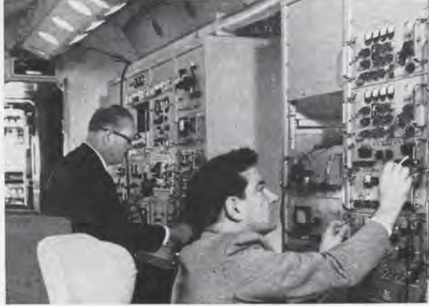
Dual-diversity telemetry receivers , built by the Vitro Corp. of America for space use, are shown in a NASA aircraft. At right are the predetection combining and recording systems that extend the receiver's signal-noise threshold and permit use of a small airborne antenna.
