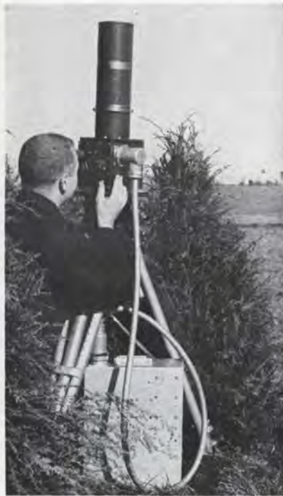
Laser range finder can measure distance of a target at night, in fog or in heavy rain. A unique memory device helps the operator pinpoint a target despite nearby clutter.
