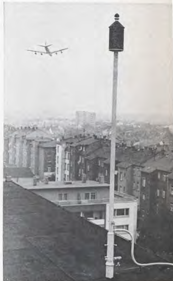
The roofs have ears in towns surrounding Frankfurt. This microphone picks up aircraft noise which is then analyzed to determine whether plane was off course, flying too low or too fast, or creating excessive noise in another way.
