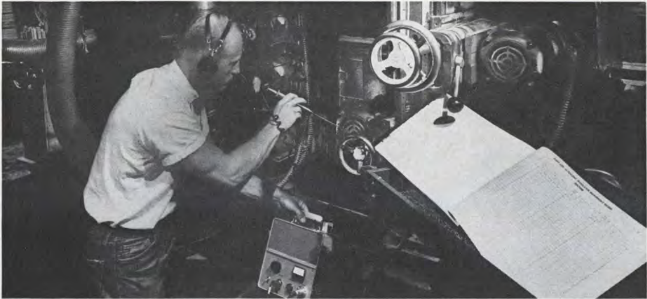
Sound analysis of machine bearings is done by translating 30-to-50 kc ultrasonic energy into audible sound in a Delcon Corp. instrument. Transistor-operated unit is applied to 42 identified probe points on bearings of wood bevel-and-tenon cutting machine, to listen for wear and plan replacements.
