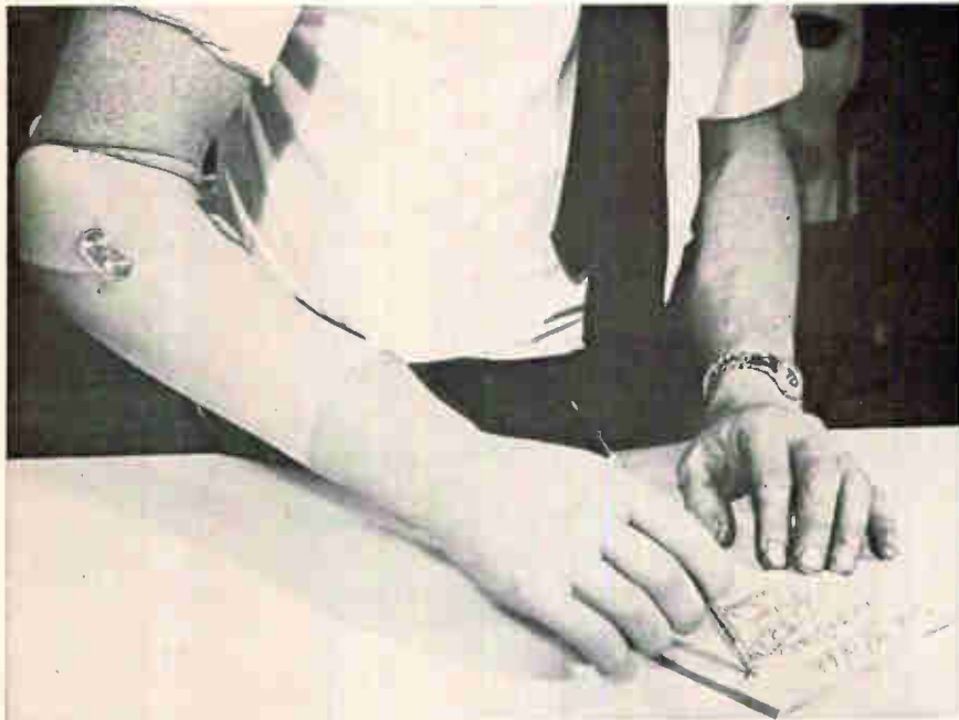
Electronic arm writes legibly after the user has had two hours' instruction and practice.
