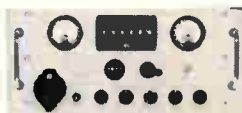
CSG Series . . . 136-138 mc in 1kc steps, 400-406 mc in 1kc steps, 1700-1710 mc in 10kc steps.
