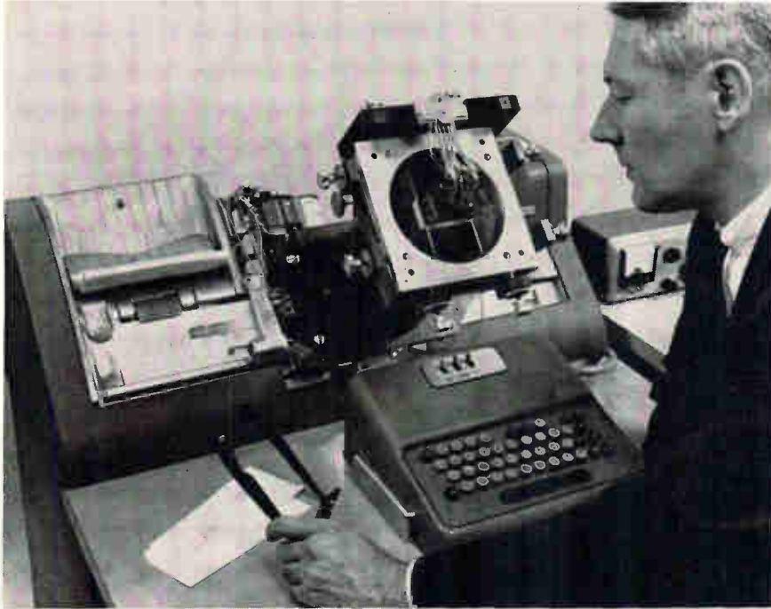
Scanistor reads handwritten numbers and letters. The experimental machine punches characters into a card as co-inventor John W. Horton looks on.
