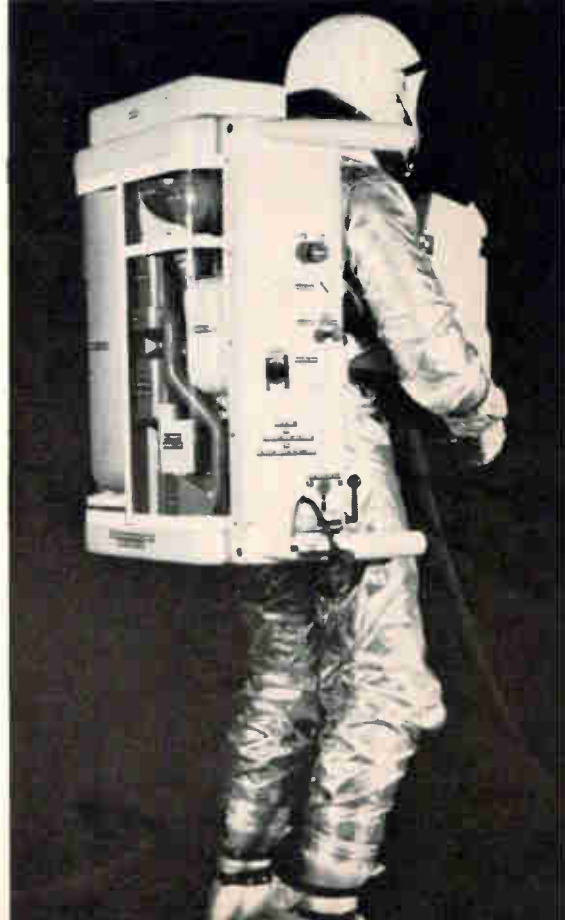
LTV "astronaut" wears a mock-up of Modular Maneuvering Unit for independent space flight.
