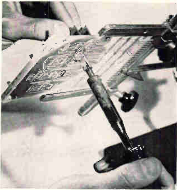
If submodule must be replaced, all the solder joints between the submodule and motherboard are melted by special tip on a soldering iron.
