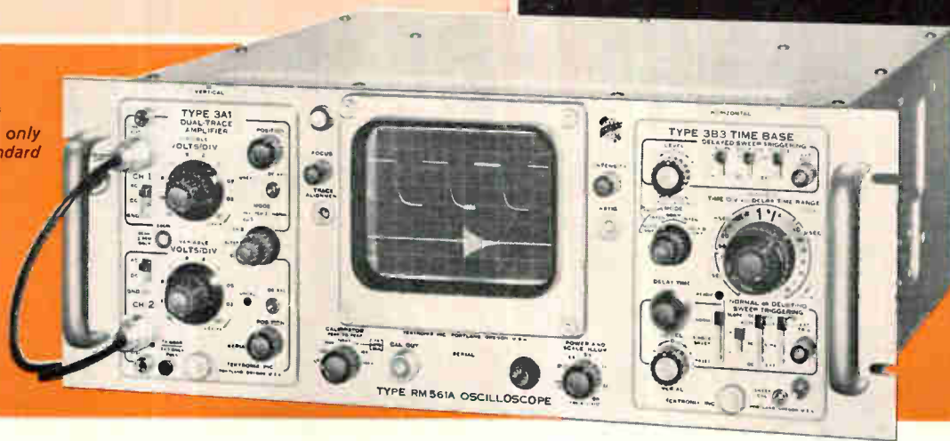
The 3A1/3B3 Plug-In Unit combination—illustrated with the rack-mount model, Type RM561A—equips the oscilloscope for high-sensitivity, dual-trace operation and sweep-delay applications.
