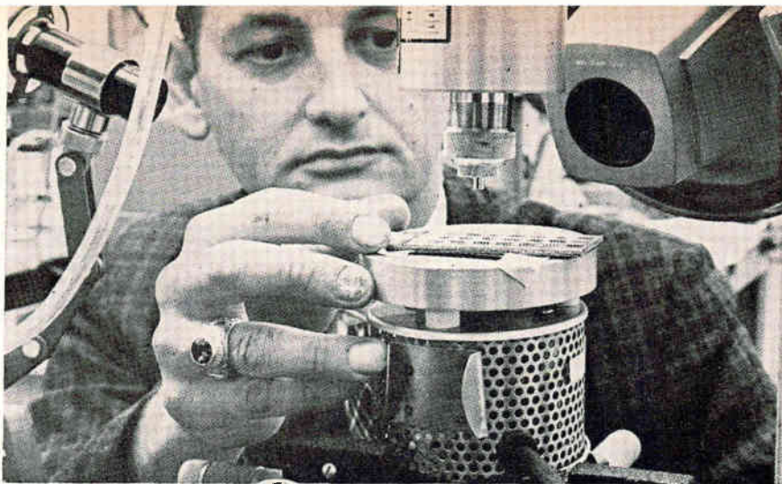
Most aerospace electronics companies are experimenting with laser welding for microcircuit assembly. This test setup at the Autonetics division of North American Aviation, Inc., uses a laser made by Hughes Aircraft Co.
