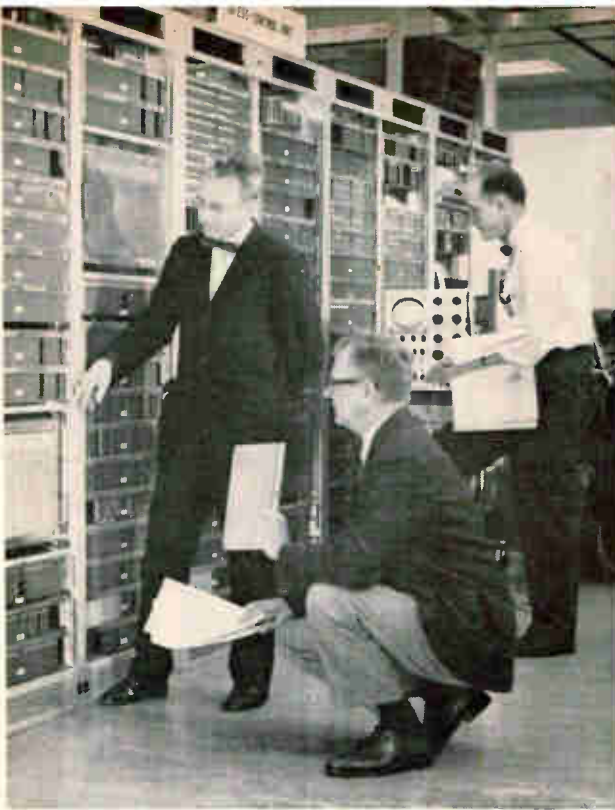
Memory unit of No. 101 ESS time-division exchange uses a twistor memory similar to that in larger offices.
