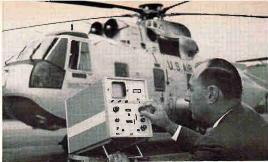
Portable instrument by Singer Metrics' Panoramic monitors noise level versus frequency on an aircraft engine during field test.
