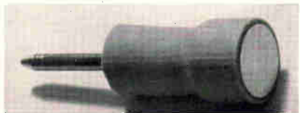
Replaceable ultrasonic cartridge attaches with a dry bond to the outside metal wall of the sensor well. The pin provides an electrical connection.
