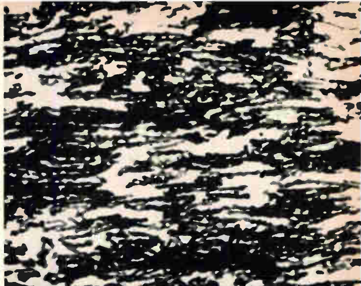
contains iron-cobalt particles made individually and then aligned and compacted into a magnet. Photos by F.E. Luborsky, General Electric Research Laboratories.
