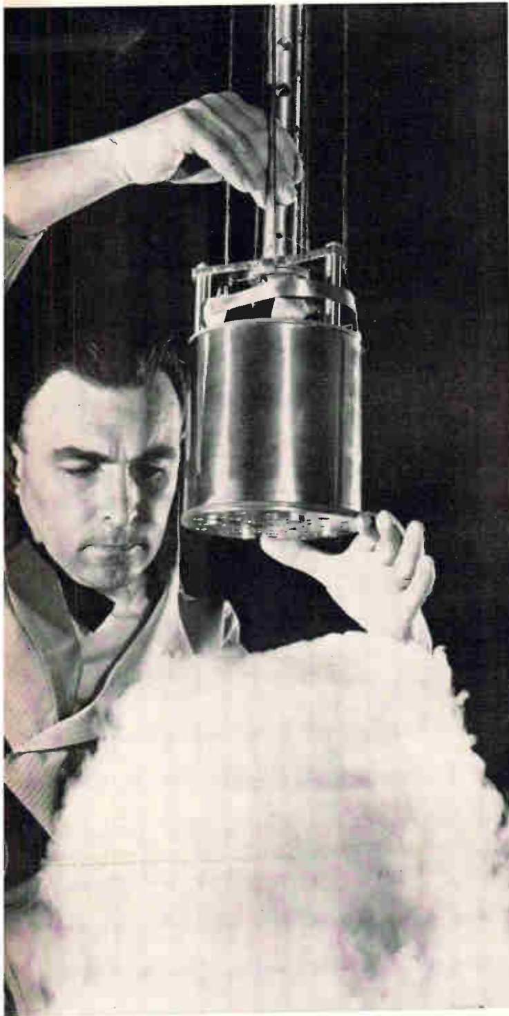
107,000-gauss superconducting magnet developed at the Radio Corp. of America's research center uses 15,370 turns of Nb 3 Sn thin-film ribbon in a compound structure (coil within coil within coil), stores 20,500 joules of energy at full field strength.
