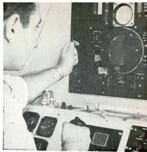
DISPLAYS for automatic TFR, built by Autonetics, consists of (center) plan position indication (PPI) and 3-D terrain to give azimuth, range and elevation information. Upper scope tells position of aircraft (circle) in relation to where automatic terrain following command (dot) says it should be
