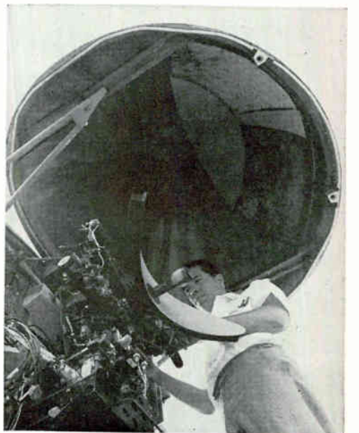
ANTENNA dish permits 90-deg azimuth scan and wide elevation coverage in automatic TFR unit built by Autonetics
