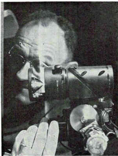
HORIZON projector generates an artificial horizon of light around pilot at all times, kept parallel to earth's horizon by vertical gyro commanding pitch and roll drive servos—Fig. 2
