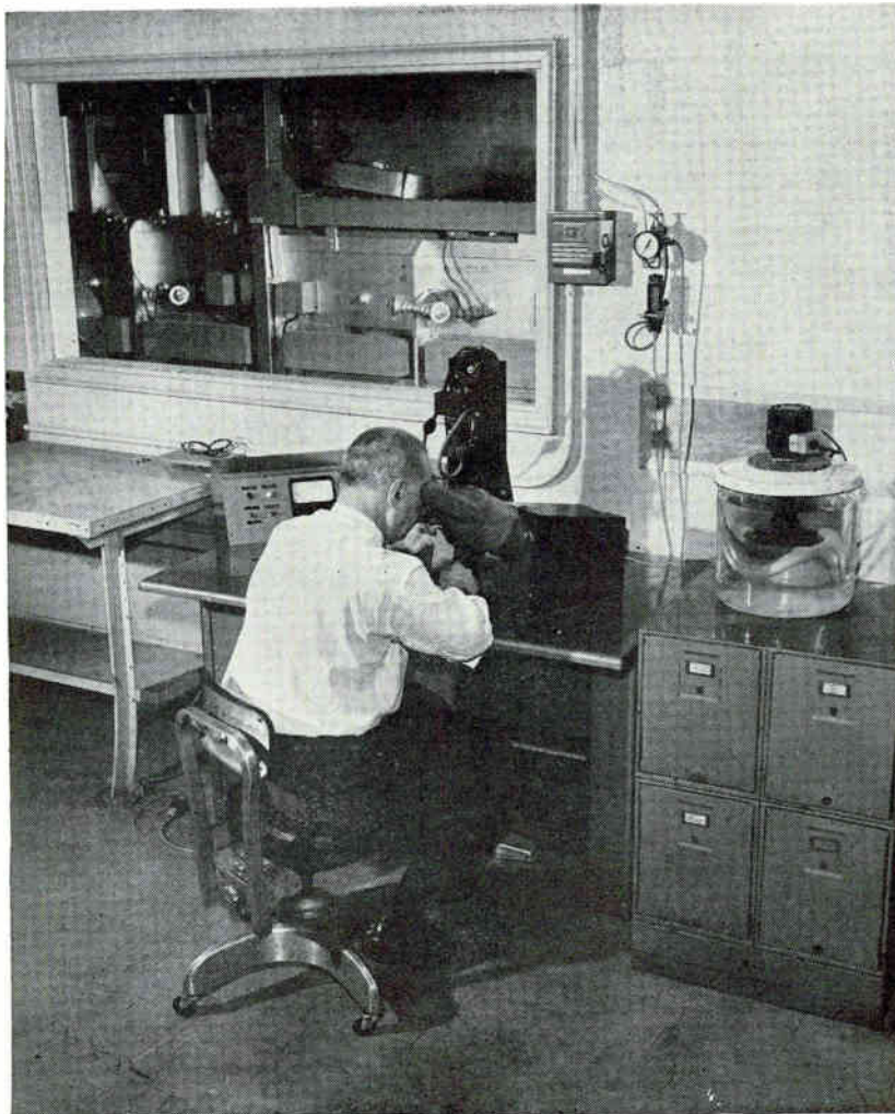
RESISTOR-TRIMMING laser has control panel operator's left, magnifier in center, and focusing screen on right. Laser head is not visible since it is located beneath the console
