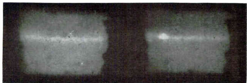
SPECTRAL characteristics of a laser at 2 deg K (top); the recorder gain is reduced between currents. Laser photographs taken through a microscope with infrared-sensitive film: below the threshold (bottom left), the light emerges uniformly from a narrow region near the p-n junction; above threshold (bottom right), the simulated emission appears to come from small spots—Fig. 3
