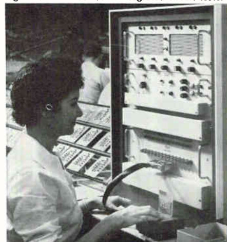
Figures 5 and 6. New welded package Figure 8. TI Model 659A integrated circuit tester
