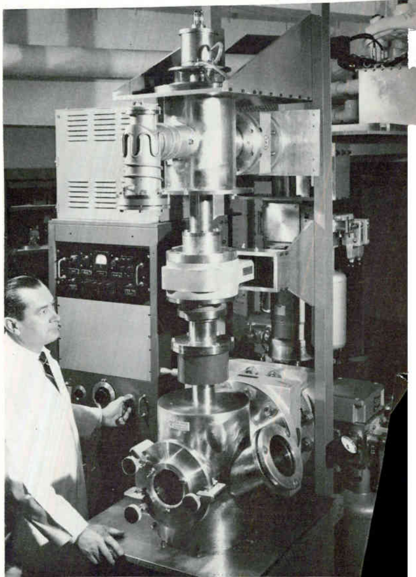
Close-up of an electron/ion and molecular beam unit used in the investigation of selective deposition methods of microcircuits.
