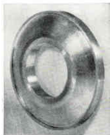
OFHC COPPER (Ring Forging, Rough Machined)
