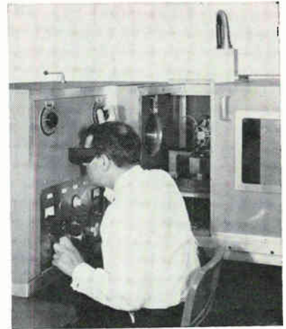
OBSERVING the changing x-ray diffraction pattern of a semiconductor crystal, Picker engineer rotates the specimen by turning vernier dial, in order to locate exact direction of crystal planes
