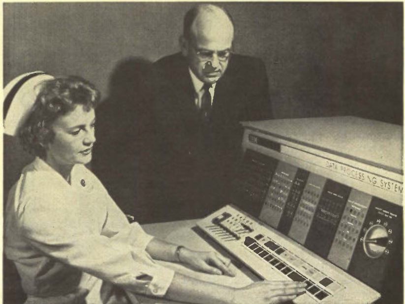
IBM 1710 computer is the heart of a hospital information system that will be installed next spring at Children's Hospital of Akron (Ohio). Terminals at nursing stations and other locations will feed patient information to the 1710, which in return will send the stations schedules for medications, diets, lab tests and x-ray examinations
