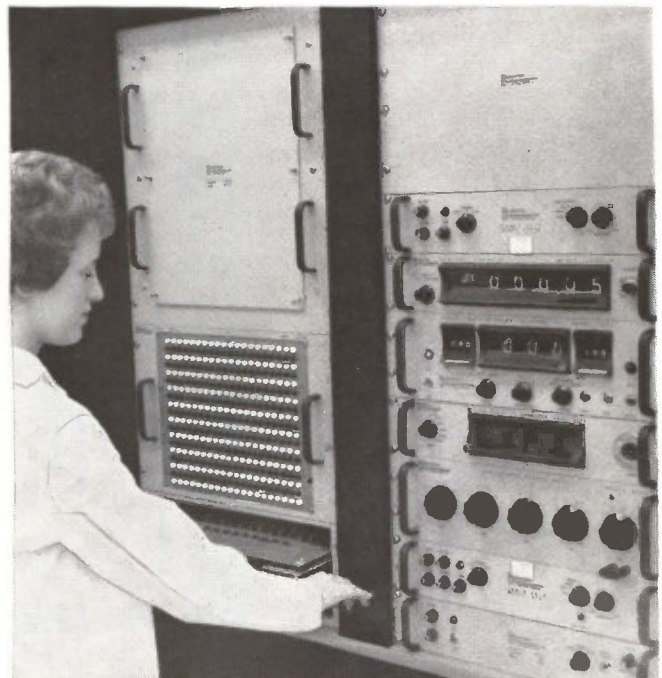
Technician at Electra Manufacturing Company inserts test resistors in the Automatic Resistor Data Logging System designed and built by Electro Instruments. Over 60 million resistor hours of data were accumulated in 18 months.
