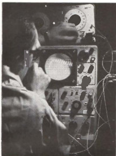
WAVEFORM carrying color information from retina of test animal to its brain is intercepted and analyzed on oscilloscope
