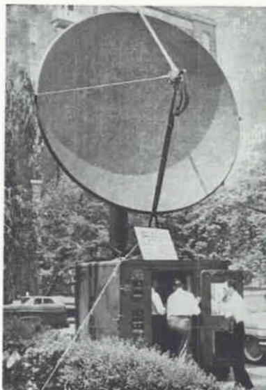
MOBILITY is emphasized in designs like the AN/TRC-66 C-band troposcatter system shown by General Instrument
