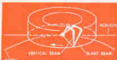
HEIGHT COMPUTER solves V-beam equation. PPI operator marks target's range and azimuth coordinates to orient acquisition gate
