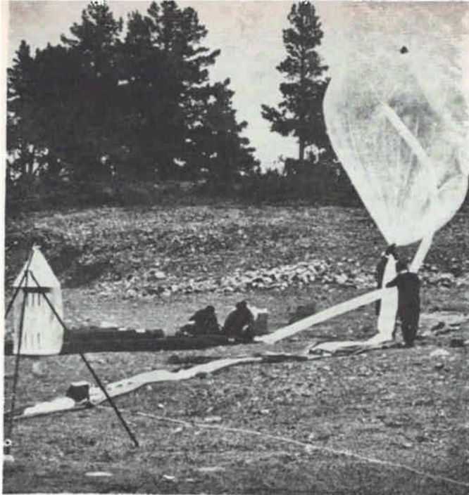
PREPARATIONS are made for balloon launching of equipment to explore x-rays and particle radiation at high altitudes in the auroral zone
