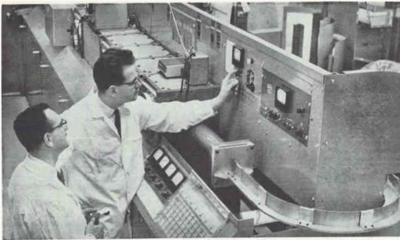
CONTROLS for setting vacuum and temperature in chambers are located at output end of machine. Diagram shows how finished substrates are returned by conveyor to storage table where substrate holders are unloaded and reloaded.
