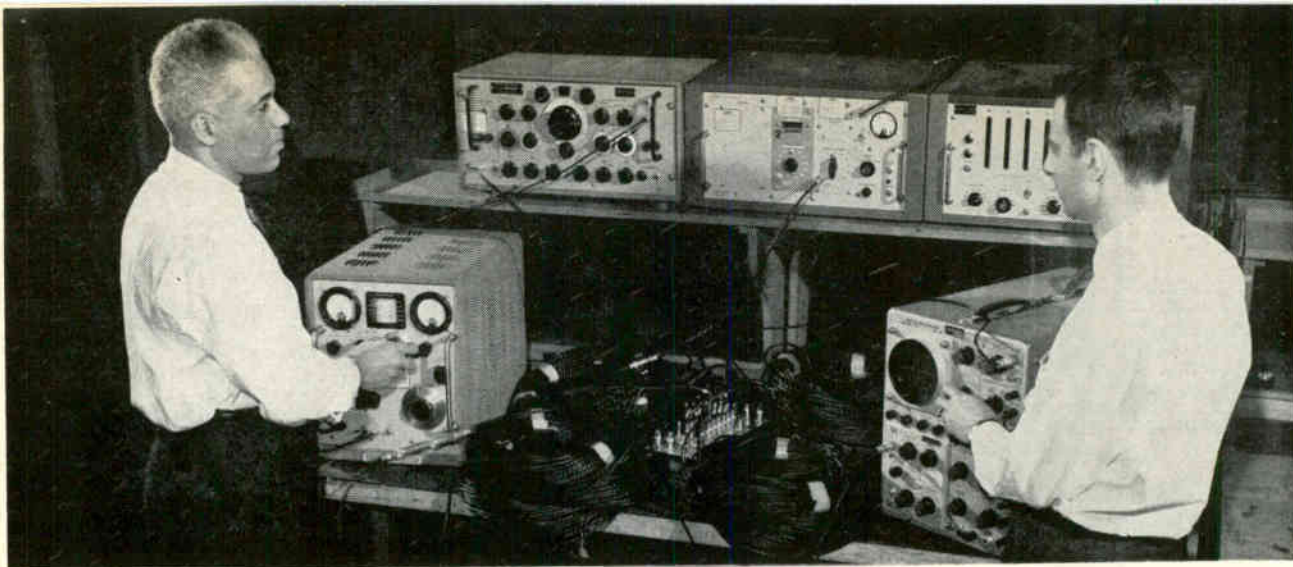
AUTHORS Morrison (left) and Sarachan test the i-f BESS breadboard model, in an arrangement that provides high resolution with an operating bandwidth of 1.25 Mc at 60-Mc center frequency. The eight pairs of coils are of slightly different lengths to provide staggered crossovers at 156-Kc intervals
