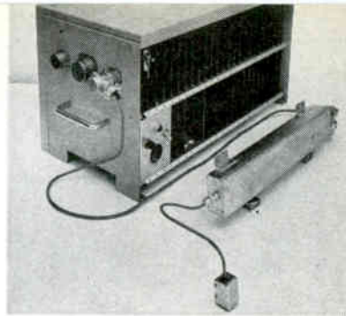
BASIC READOUT equipment is reading head (foreground), preamplifier and recognition circuits
