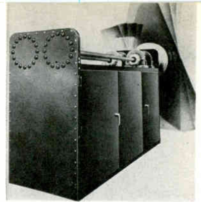
ANTENNA drive mounted on cabinet of glide-slope radar
