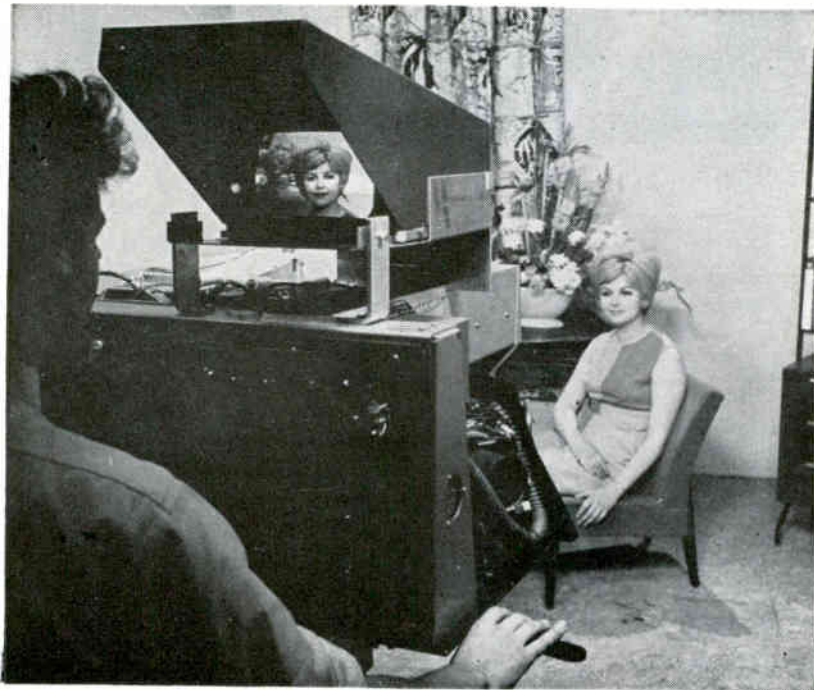
COLORFUL young lady in multicolor dress is used by Marconi during London demonstration of new separate-luminance color-tv camera. Marconi says camera is suitable for NTSC, SECAM and PAL systems. It uses three 4\frac{1}{2} -inch image orthicons, for luminance, red and blue signals. Green is derived from these three signals
