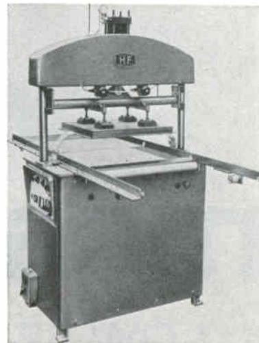
OPEN-SPAN welding press uses electrical and pneumatic circuits for positioning weld material
