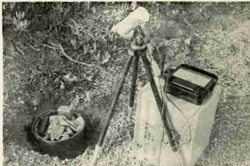
SIMULATED MINE was plastic bucket containing metal objects, fabric and fertilizer. Infrared detector, amplifier and readout meter shown at right—Fig. 1
