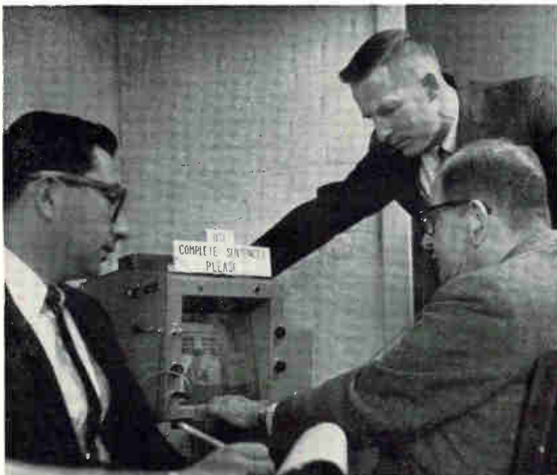
VICTIM of aphasia, language impairment due to brain injury, works teaching device developed at University of Michigan while two researchers look on. Machine helps patient regain normal speech by asking him tape-recorded questions about pictures it presents
