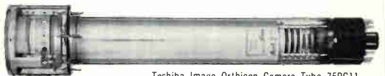
Toshiba Image Orthicon Camera Tube 75PC11
