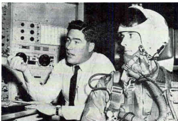
B-58 ecm simulator, already in operation over a year, provides space for instructor not available in airborne training
