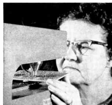
TINNED COPPER PINS replace eyelets in machine connection technique
