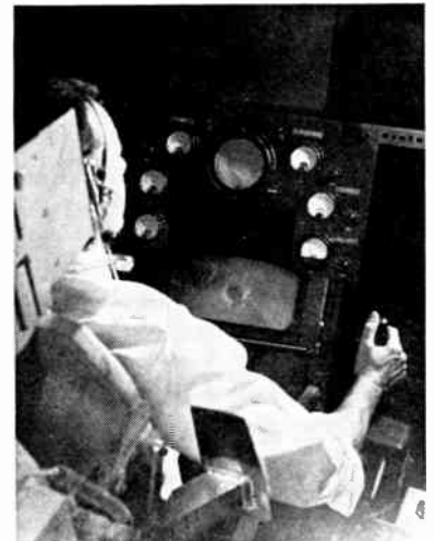
LANDING simulator, one of four built by Boeing to study space flights, uses tv to project relief map of moon and an analog computer to simulate spaceship operation
