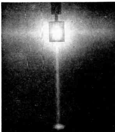
SELF-COLLIMATED electron beam from a perforated hollow cathode in helium—Fig. 1
