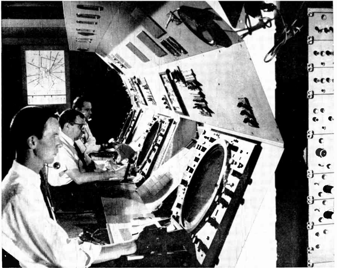
REMOTE SITE displays for Texas Instruments ASR-4 offer operator choice of three modes of video presentation: normal radar video only, moving-target indication or both
