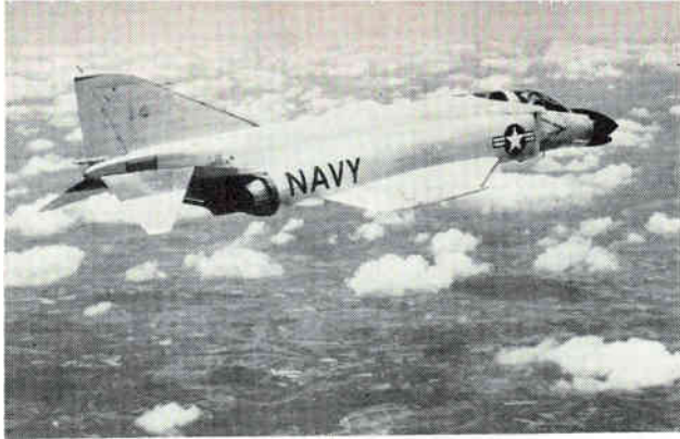
NAVY'S F4H Phantom II is equipped with electronic detection gear, an all-altitude bombing system, and once set a speed record (1,390.31 mph) for the tight, circular 100 Km closed course
