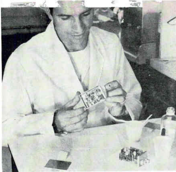
TINY BEACON is about the same size as a package of cigarettes and is encapsulated for improved mechanical stability and protection
