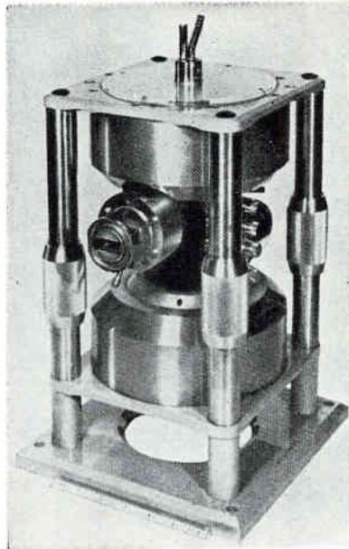
Doppler radar water-cooled klystron in focusing magnet assembly
