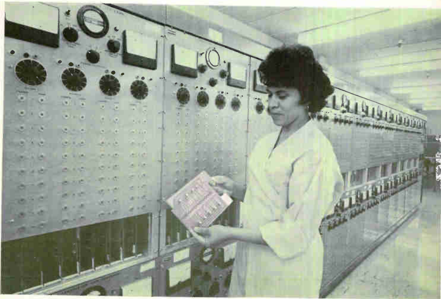
RELIABILITY test of transistors at Raytheon's Mountain View, Calif. plant
