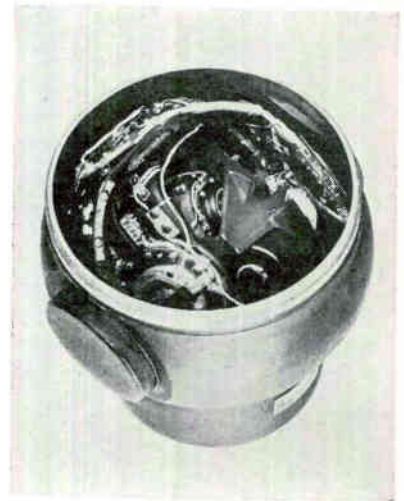
INERTIAL vertical reference, capable of holding a camera platform within 0.05 second of arc per second of time. System operates as a Schuler-tuned pendulum, uses brushless torque motor
