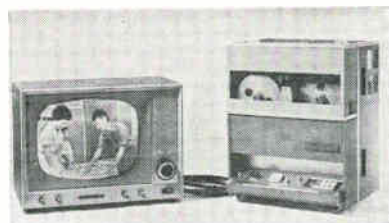
VIDEO recorder slightly larger than tv set has been announced by Sony. Tape, with audio, video and synchronization tracks, can be played back at 1/60 of normal speed
