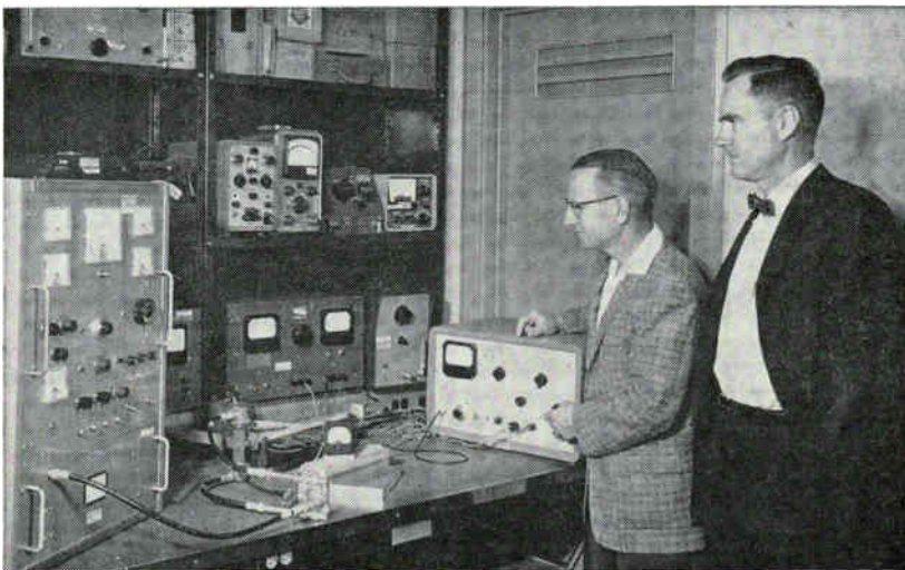
AUTHORS Lundquist and Strother measure noise figure of balinverter. The converters used are Sage Laboratories model 242 coaxial single-ended mixers
