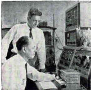
PROPERTIES of crude oil in refinery process stream are compared with those of reference sample in paramagnetic resonance analyzer
