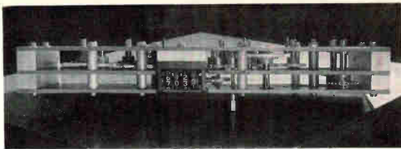
GEAR PLATES, made from aluminum filled epoxy, work well for normal temperature range but thermal expansion can cause trouble if temperature variation is too wide.
