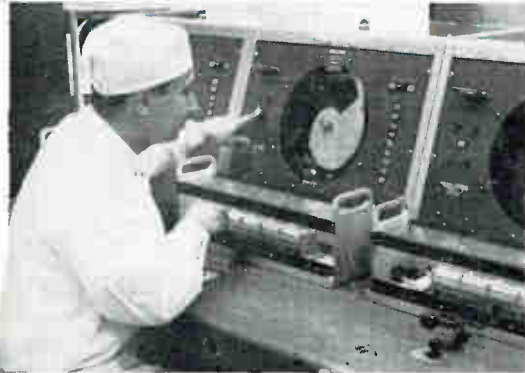
Automatic magnetization and stabilization eliminate operator variability, ensuring required field characteristics.
