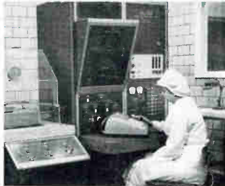
All helices are inspected to a tolerance of \pm 2 microns on a Helix Pitch Error Resolver.
