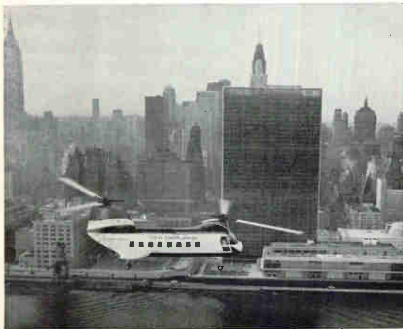
COMMERCIAL VERSION of Boeing 107 Helicopter using a stability augmentation system will be modified for Air Force long-range logistics
