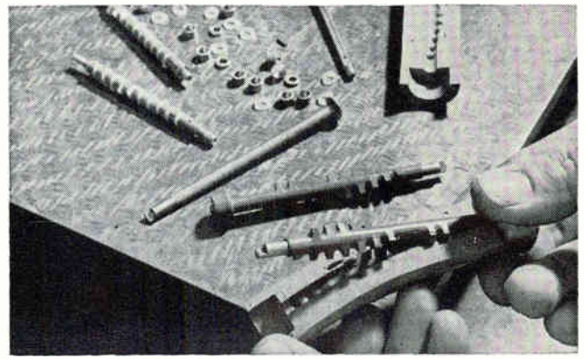
EPOXY CAM SHAFTS with cam heights held to \pm 0.001 inch are molded on knurled center shafts instead of using nylon cams on flattened shaft. Molds were cast from a cold pouring silicone rubber
