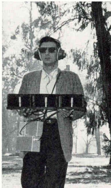
ECHOES of supersonic signals transmitted and received by transducers in box are heard in ear-phones
