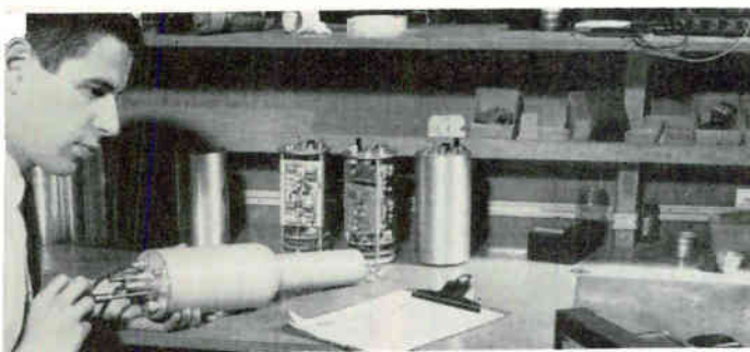
RADIATION DETECTOR differentiates between two types of nuclear particles by distinguishing between their different energy levels. It is being adjusted at the plant of Nuclear Enterprises in Winnipeg
