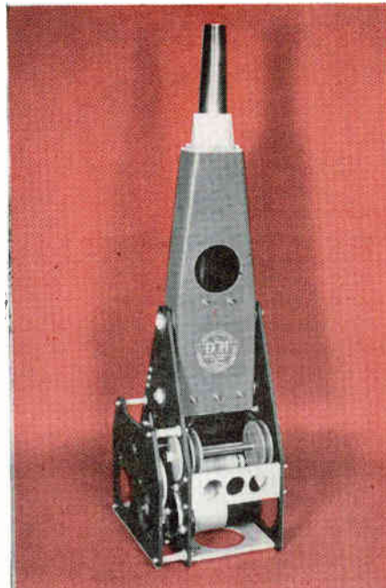
RETRACTABLE ANTENNA UNIT. Antennas of this type are used in the U.S. Gemini program, and in Canada's own Topside Sounder satellite. The mechanism unreels a steel tape into a rigid tubular antenna up to 75 feet long. DeHavilland Aircraft of Canada, Ltd, Malton
