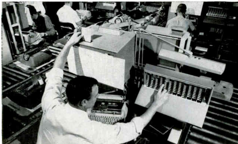
Computer-based quality control system in use at IBM's typewriter plant in Lexington, Ky. Factory Data Collection System feeds punched-card inspection data to Rmac data processor. Computer immediately reports abnormal defect levels and also prepares daily and weekly analyses
