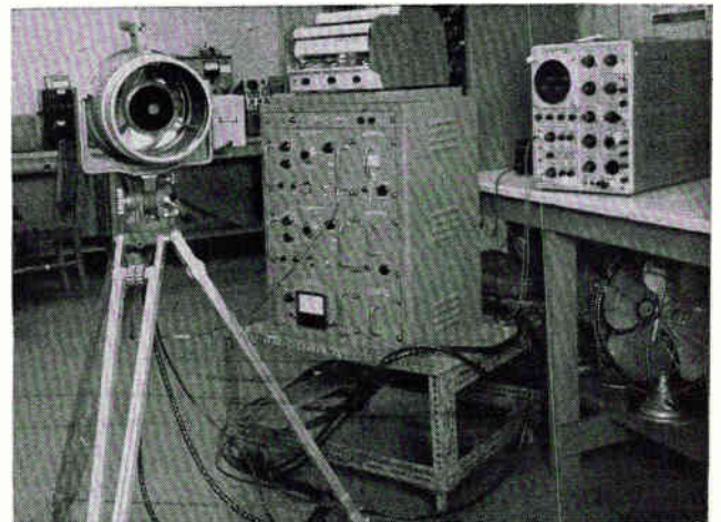
INFRARED CAMERA (left) showing adjustments (but not electronic circuits) and light sensitive camera back. Radiometer and electronic circuits (right) with recorder
