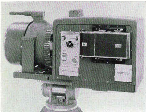
INFRARED CAMERA (left) showing adjustments (but not electronic circuits) and light sensitive camera back. Radiometer and electronic circuits (right) with recorder
