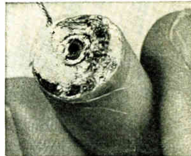
Lead is attached to capacitor with bonding technique
