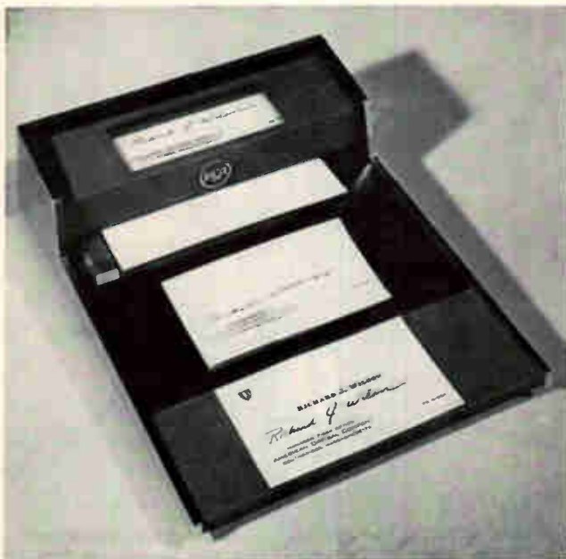
FIG. 10—Signa-Guard optical decoder, for signature protection in banks, uses fiber optic scrambler, (left); a thin fiber shows waveguide power transmission modes, (right)
