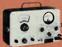
Solid State Model 127 A-Y Special feature: Solid state with rechargeable battery pack. Carrier rack fast patch for use with Western Electric Type O and N carrier Frequency range: 2 KC to 350 KC Selectivity: 250 cps Frequency accuracy: \pm 1 KC Measuring accuracy: \pm 1 db Size: 7½" x 7½" x 12½", 16 lbs., including batteries Price: $945.00 with battery pack. Rechargeable batteries and charger optional at extra cost
