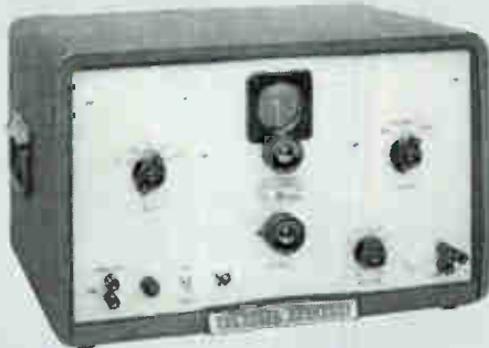
⚡ 202A Function Generator, 0.008 to 1,200 cps.
