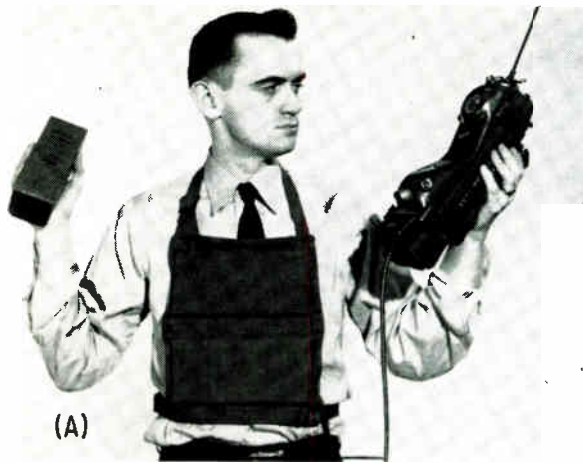
FIG. 2—Vest battery for radio set AN/PRC-6 (A). External (B) and internal (C) views of automatically activated zinc-silver oxide battery used in many missiles
