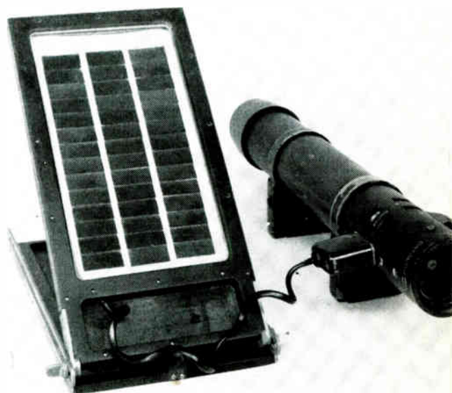
FIG. 5—Experimental solar powered battery charger for photoflash gun
