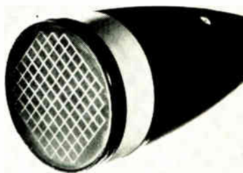
Corning uses photosensitive glass to form graticule inside the glass viewing surface of crt
