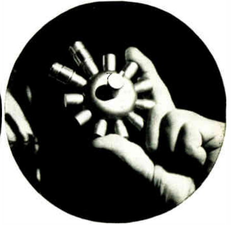
Radical design of Raytheon Amplitron, which has single magnet, cuts weight to 16 oz. It delivers 25 watts at S band, has 60 percent efficiency
