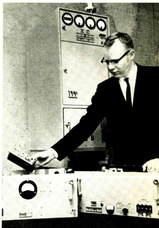
Engineer holds exciter-multiplier module of ITT S or C band transmitter. Compact, solid-state, 1-Kw system has only one tube, a klystron
