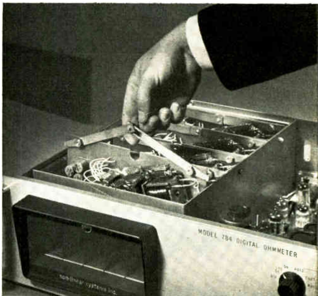
Both the 484A and 784 feature plug-in stepping switches.
