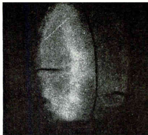
Kerr cell photo of electrodeless plasma accelerator at Institute of Physics, Uppsala, Sweden, shows plasma ring traveling from right to left at 5 \times 10^6 cm/sec. Exposure time is 10^{-7} sec
