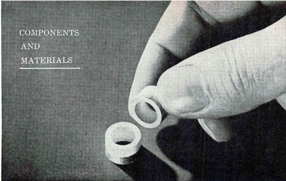
Beryllia cylinders have thermal conductivity greater than cast aluminum, very low loss tangent at microwave frequencies. Significance: Cement cylinders into power transistors to operate at power ratings required, forget weight and size hitch
