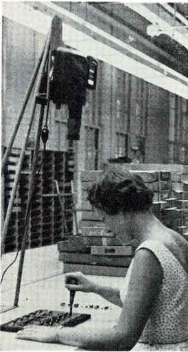
Projector mounted on tripod gives assembler a one-to-one image of the assembly
