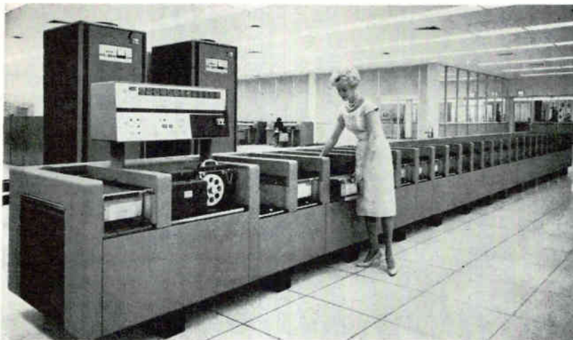
Checks, packaged in plastic jackets and identified by coded magnetic tape strips, are sorted into preprogrammed groups. Unit is part of ITT Corp. automated system for processing bank documents
