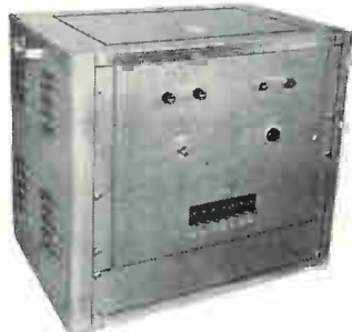
ABOVE — STATIC POWER RECTIFIER Output: 500 KW, 500 volts DC 1000 amperes Input: 13,800 volts, 33 amp, 3 phase, 60 cycle
