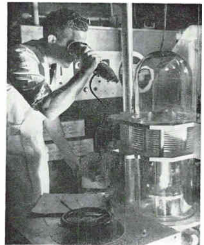
Optical pyrometer is used to check temperature of subassembly during vacuum firing
