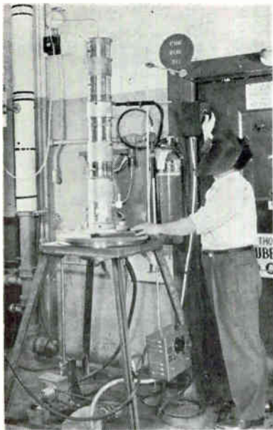
Klystron is Heliarc welded on motor driven turntable
