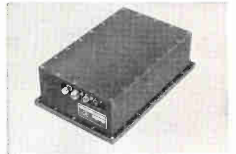
Microdot model 2406A UHF Telemetry Transmitter, similar to units now in production for the Midas satellite program.
