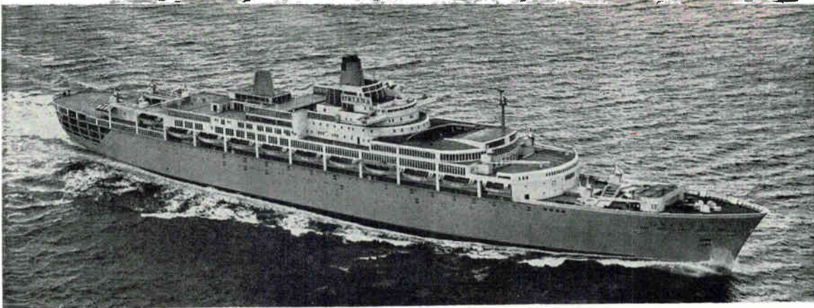
The T.S.S. Oriana, on which the power meter is used. The 42,000-ton liner develops 40,000 horsepower per shaft at 157 rpm. Meter measures torque of about 600 tons-feet on 96 feet of a 25-inch diameter shaft. Ship's top speed is 31 knots
