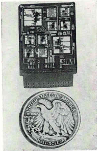
Microelements of reversible binary counter are set flush on plug-in card (left). Components performing same function are shown in larger system (right) that uses miniature building blocks
