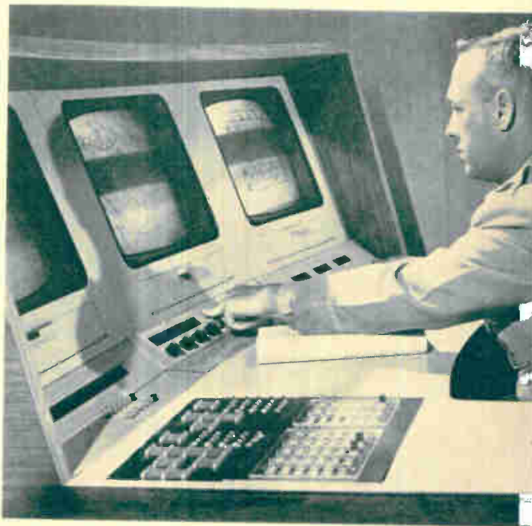
Master control console at Air Force Satellite Test Center monitors Discoverer, Midas and other military polar orbiting satellites, was built by Radiation, Inc. for Lockheed
