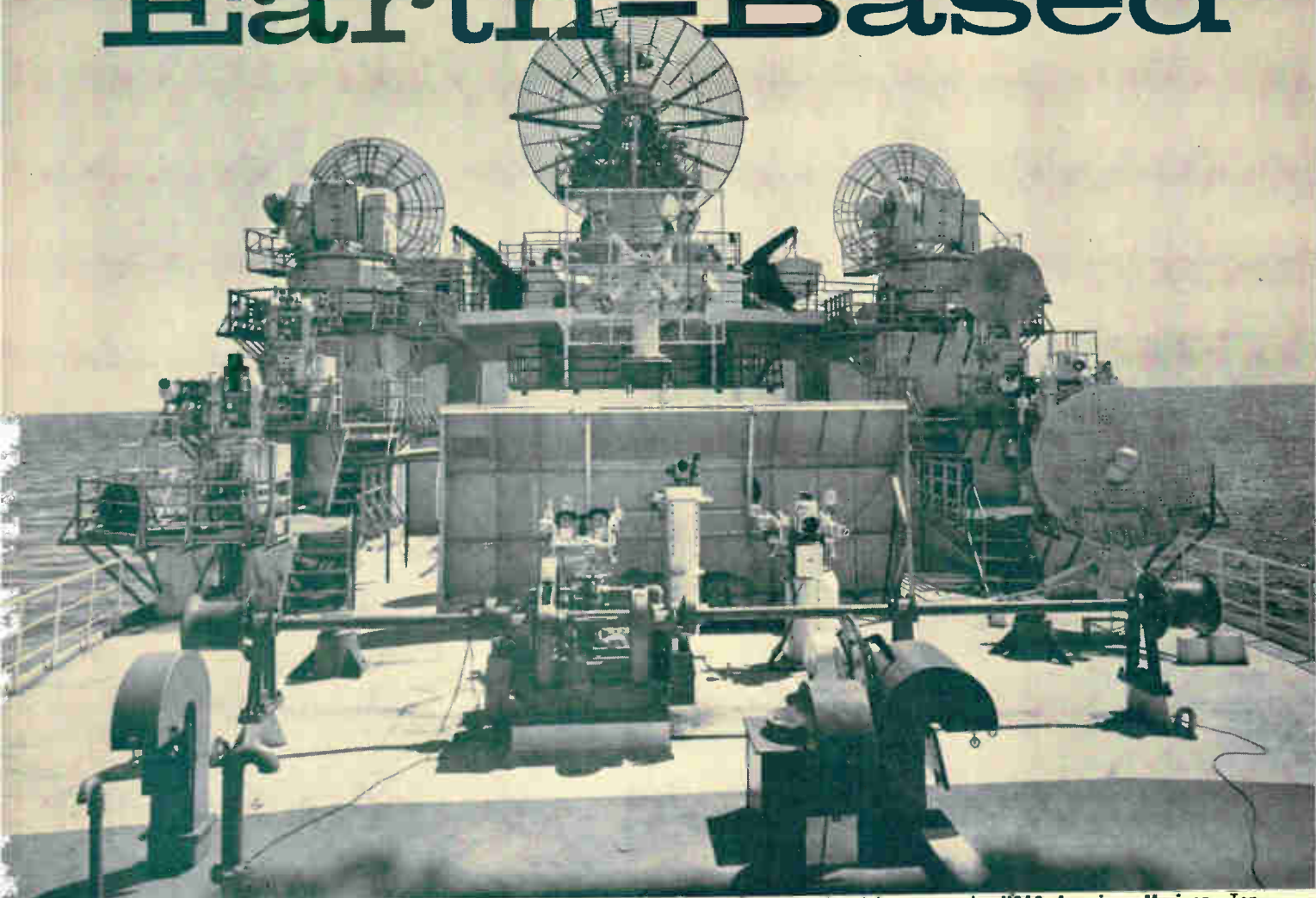
To discover a missile's vulnerable points they are studied on reentry by a floating laboratory, the USAS American Mariner . Top center is a uhf L-band antenna and on either side, C-band tracking radars (RCA). Below are optical instruments (Barnes Engineering) that cover the spectral region from the far ir through uv. Downrange Antimissile Measurement Program is sponsored jointly by the Army Rocket and Guided Missile Agency and the Advanced Research Projects Agency
