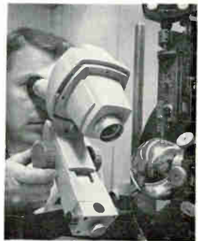
Diamond stylus scribes surface of spherical rotor for gyro
