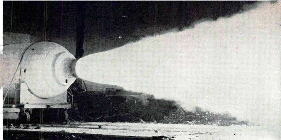
At McGregor, Texas, Rocketdyne test fires at -75^{\circ}\text{F} a rocket motor containing 3,500 lb of solid fuel
