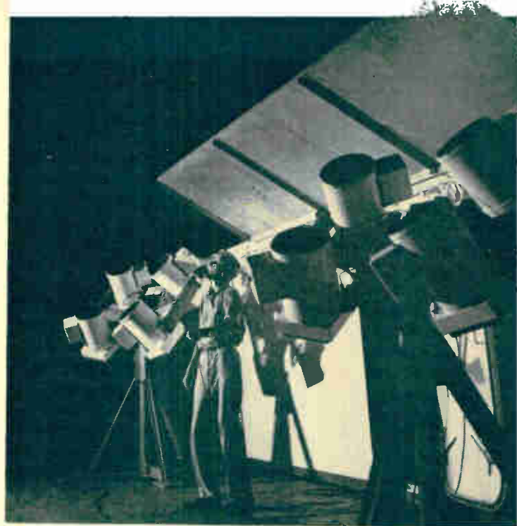
Two ballistic camera arrays record missile reentry from the deck of USAS American Mariner . Such systems, land-based and ship-based, will continue to play important role in missile range facilities (Barnes Engineering)
