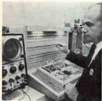
North American Aviation designs aircraft and space ship cockpit instruments with this device. Varying connections creates different images of instruments on the oscilloscope display tube, allowing engineers to experiment with instrument face design
