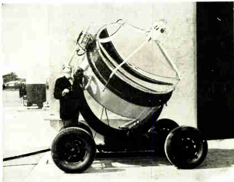
Solar concentrator mounted on aircraft searchlight housing is tested with cryogenic calorimeter. Thompson Ramo Wooldridge Inc. developed unit for Air Force as part of thermionic power system
