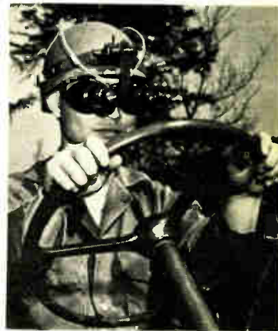
Infrared binoculars for night viewing are under development at the U. S. Army Engineer R&D Laboratories, Fort Belvoir, Va. The optical system utilizes an infrared converter tube
