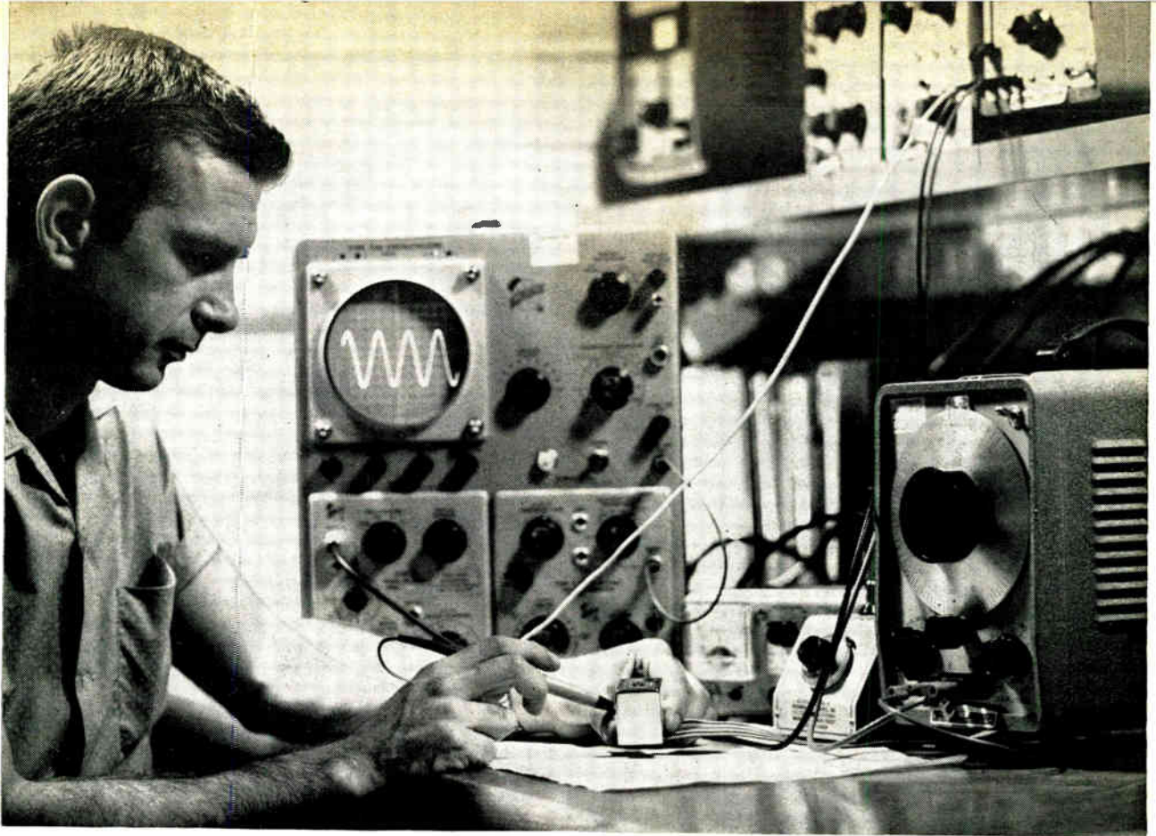
The low-drift transistor d-c amplifier under test. To alleviate temperature problems, differential amplifier uses a pair of matched transistors in one can
