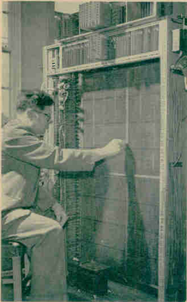
Fixed ferrite memory of a Ferranti high-speed computer under test in England
