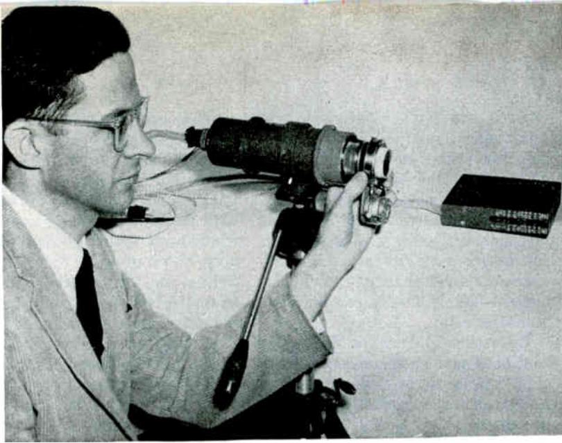
Typical slow-scan tv transmitter with mechanical shutter attached to lens weighs 6 lb and occupies 80 cubic inches
