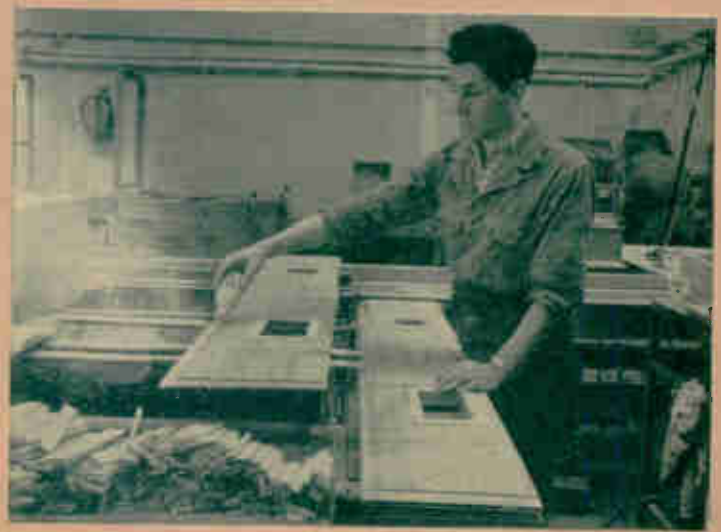
Waxcoating sets glue fast in Van Der Helm tv cabinets: Glue is applied to unwired part . . .
