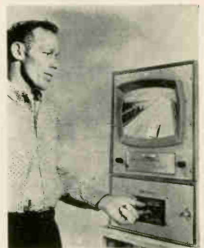
Closed-circuit, wide-angle television by GE aids operator in Chicago to watch other side before raising bridge
