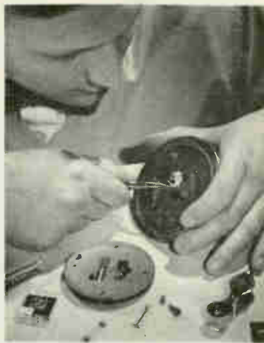
Evaporation mask containing amplifier circuit is etched on machine (left). The 0.005-in thin steel sheets containing masks for the passive elements are then mounted on evaporation fixtures (center). After conductance resistance and capacitance elements are deposited on the substrates by high-vacuum techniques, micromanipulator (right) is used to mount the active elements on tiny thumbnail-size circuit (below)
