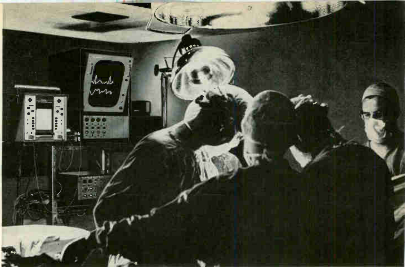
Sanborn's monitoring system displays physiological condition of patient to surgeons throughout operation. Seventeen-inch oscilloscope shows an electrocardiogram (top) and a sphygmograph (bottom)
