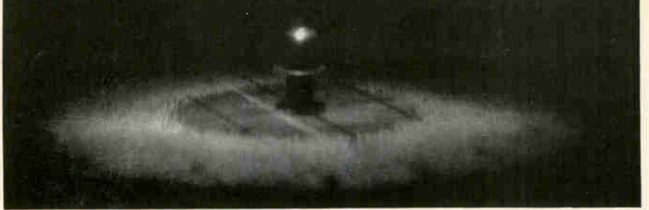
High-speed underwater photo of transducer, showing cavitation on the aluminum disk during the back phase of motion
