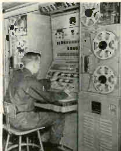
Mobidic, mobile digital computer developed by Sylvania, will be used by Seventh Army in Europe
