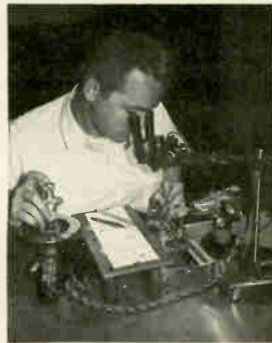
Evaporation mask containing amplifier circuit is etched on machine (left). The 0.005-in thin steel sheets containing masks for the passive elements are then mounted on evaporation fixtures (center). After conductance resistance and capacitance elements are deposited on the substrates by high-vacuum techniques, micromanipulator (right) is used to mount the active elements on tiny thumbnail-size circuit (below)
