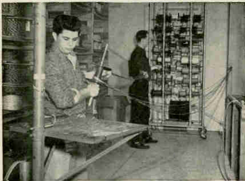
Trimming end of wire bundle
