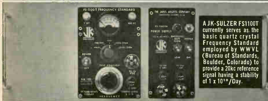
Total Dimensions, Standard and Power Supply: 7½" W x 6" H x 12½" D. Shown mounted in 7" x 19" rack panel.
