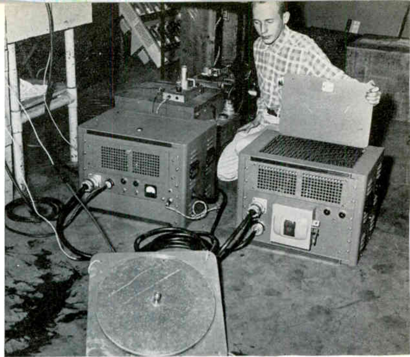
Sonar thumper. In foreground is transducer, with aluminum plate resting against epoxy-encapsulated coil. When 0.1-ohm coil is energized, motion is about \frac{1}{2} inch in water. Background: capacitor bank and trigger (l.), power supply (r.)
