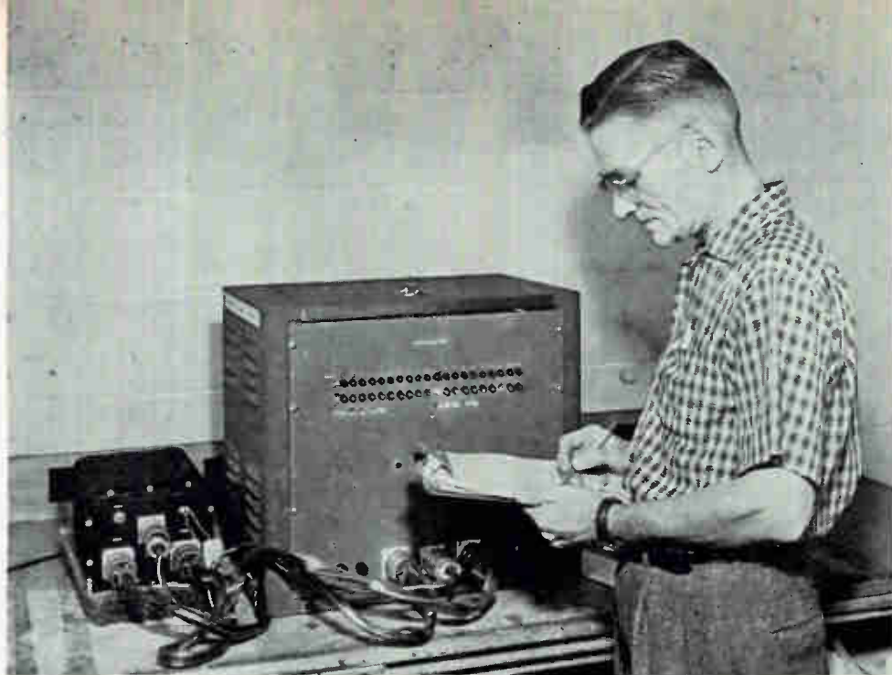
Automatic relay tester monitors 20 normally closed and 30 normally open contacts in the equipment at left. Toggle switch S_1 is hidden by the clipboard. Reset pushbutton S_2 is at the lower right of the panel
