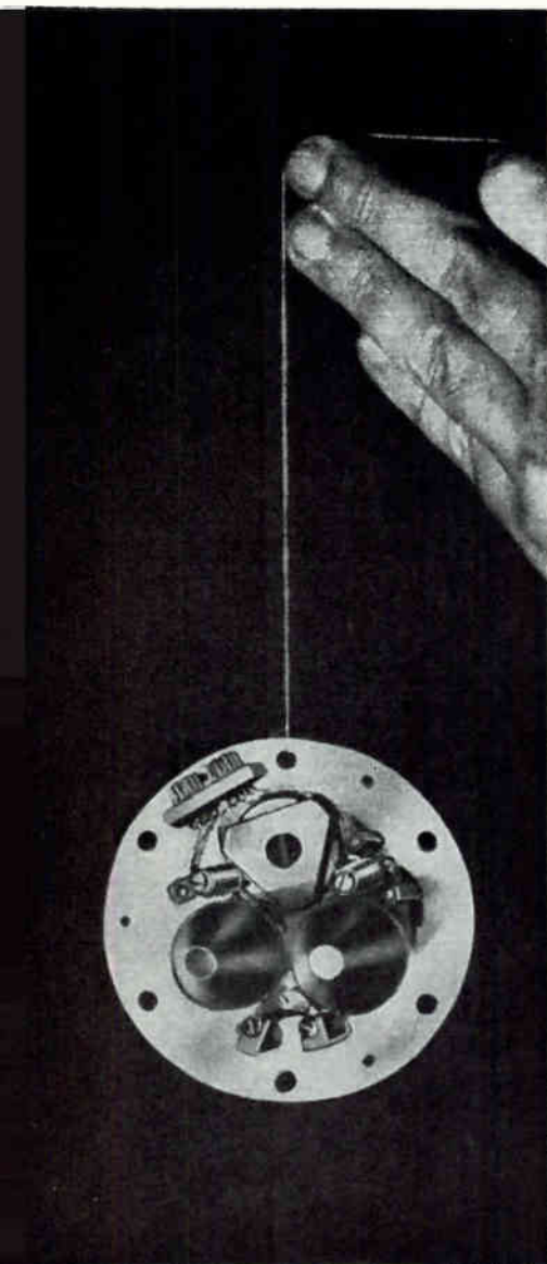
Two-channel infrared radiometer weighs 1½ oz, operates on 50 microwatts
