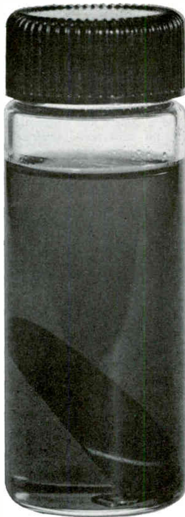
ORDINARY CHLORINATED SOLVENT under same conditions dissolves resin, damages metal.
