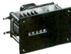
Series 1606/mechanically actuated manual reset standard; bi-directional (non-reset) available. Speed 5000 cpm, up to 5 figures
