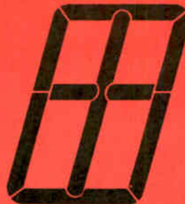
SYLVANIA TYPE NU-150 . . . 1½" NUMERIC . . . is dia- gramed above in actual size to show the 9 segments that produce a display of 0-to-9 numerics.
