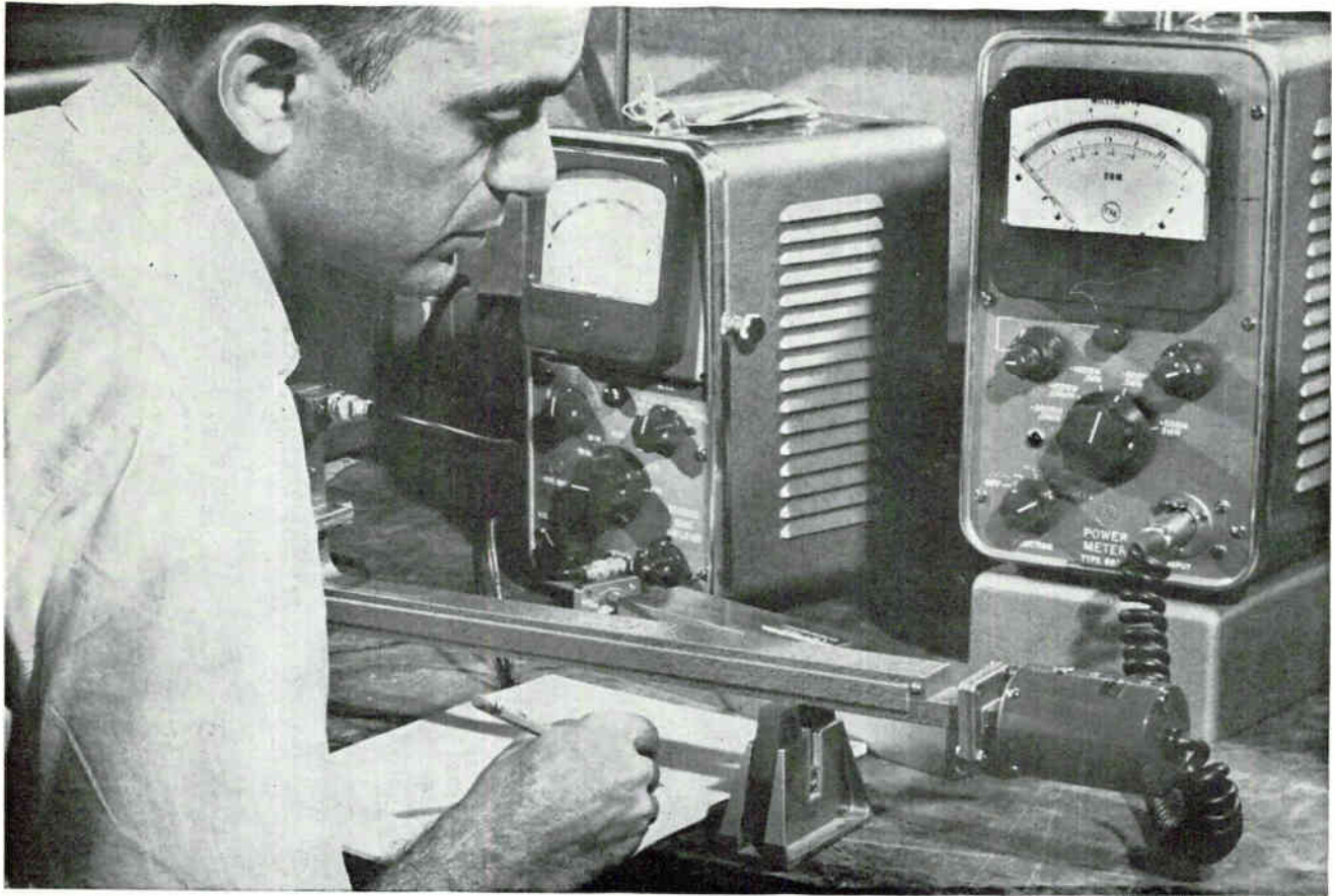
Temperature compensated power measuring unit connects to waveguide by flange mounting plate
