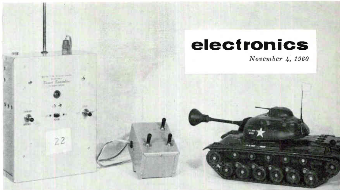
FIG. 1—Scale model tank and transmitter simulates operation of actual medium tank. Tank cannon houses light-beam gun used to kill other tanks
