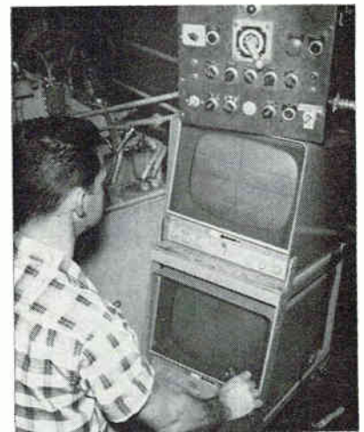
Picture enables operator to bore-sight tack rivets used as tape-to-panel synchronizing points when Drivmatic Riveter at Douglas Aircraft is operating automatically
