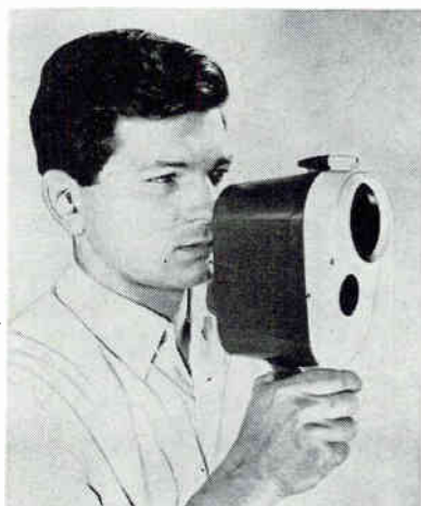
Communications device developed by Infrared Industries, Inc., uses infrared radiation as voice carrier
