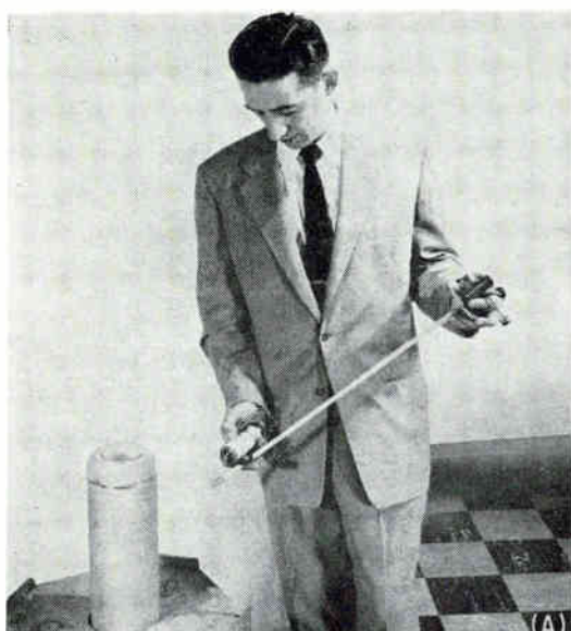
FIG. 2—Millimeter-wave maser (A) developed at Lincoln Lab uses a small superconducting electromagnet (shown in right hand of author). Details of maser cavity and cross-section of low-temperature dewar with maser in place are shown in (B). Active material is dark area at end of dielectric slab, which almost completely fills cavity
