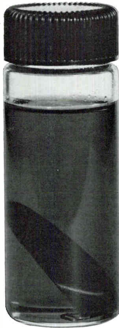
ORDINARY CHLORINATED SOLVENT under same conditions dissolves resin, damages metal.
