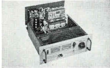
"Flip Top Box" Permits Accessibility For Maintenance
