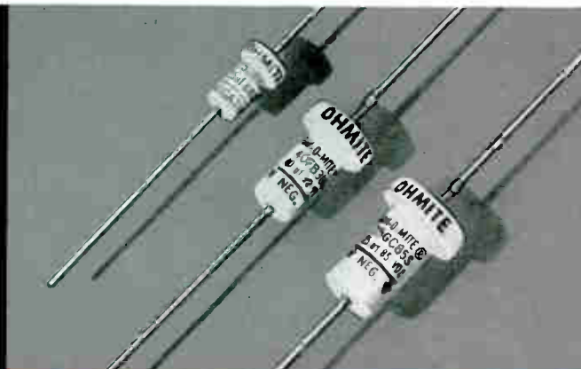
ALL THREE CASE SIZES of "hatted" capacitors—U, F, and G
