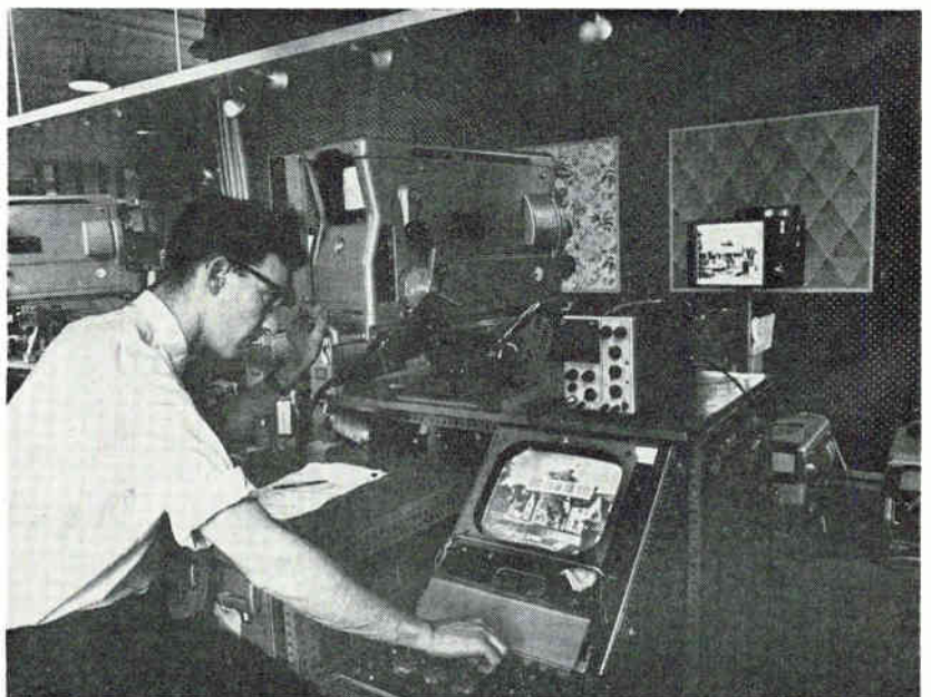
Warsaw's new Marconi Mark IV television camera (above) is compatible with USSR standards—625 lines, 50 fields, eight Mc/s channel
