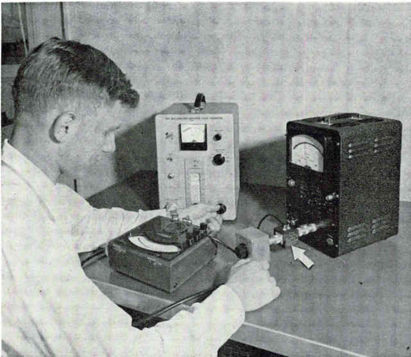
Engineer makes use of micropotentiometer (arrow) to calibrate a new vtvm soon to be marketed by Ballantine Laboratories
