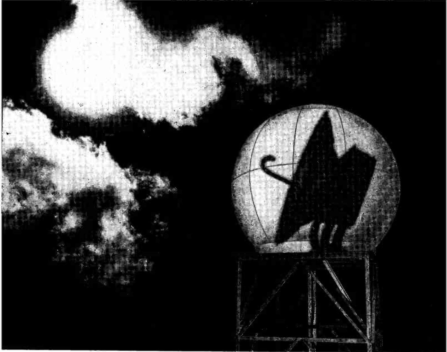
Eighteen-foot diameter radome of WSR-57 Stormfinder radar. System operates at S band, has 250-mile range.
