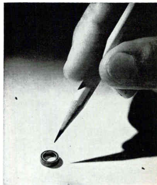
Doughnut-shaped artificial neuron by Ford's Aeronutronic division duplicates human nerve
