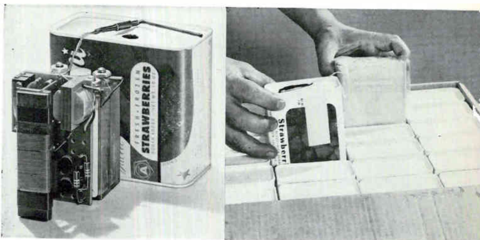
Physical layout of complete temperature-sensitive transmitter (left); a transmitter is readied for operation with its temperature-sensing probe inserted in an adjacent carton of strawberries (right)
