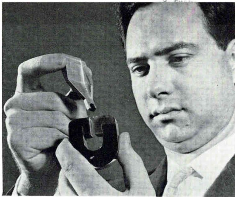
Half-inch-square synthetic ruby maser at tip of copper transition section held above 12-oz magnet by T. H. Maiman of Hughes Aircraft
