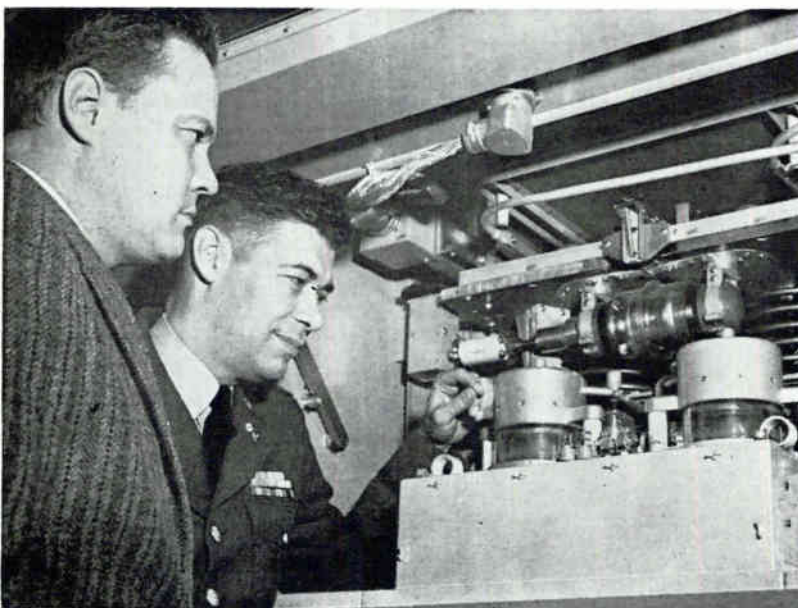
Prof. Von R. Eshleman and Lt. Col. R. C. Barthle inspect 40-Kw Collins transmitter that sent radar signal to sun and back in Stanford University experiment
