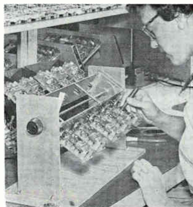
Revolving fixture for plug-in unit assembly
