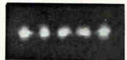
Firing of bank airgap switch, improper adjustment
