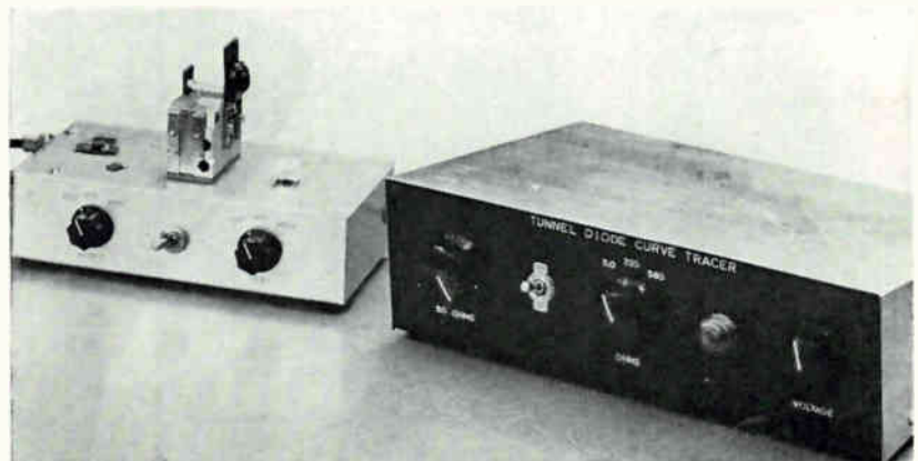
Diode holder and amplifiers are separated from power supply and sweep generator
