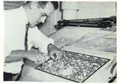
Component layout guides preparation of circuitry master
