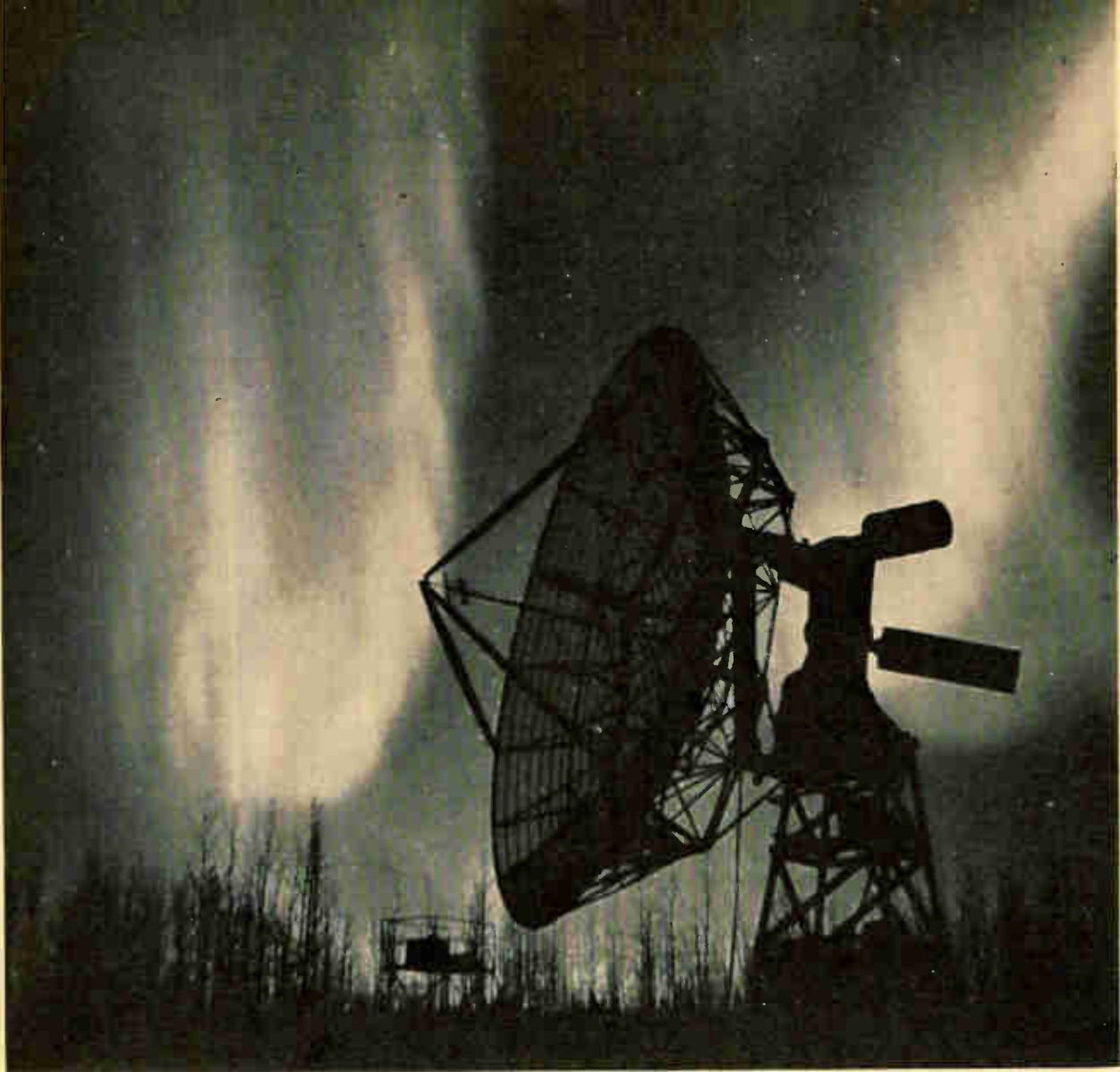
Radio interferometer used by the Geophysical Institute at the University of Alaska consists of two 28-ft. telescopes on polar mounts for tracking the circumpolar radio stars in Cassiopeia and Cygnus. Equipment operates simultaneously on 223 and 456 Mc to determine the amplitude and angular scintillation of the stars due to variations in the ionosphere. Increased scintillation has been observed during magnetic storms and auroral displays 17
