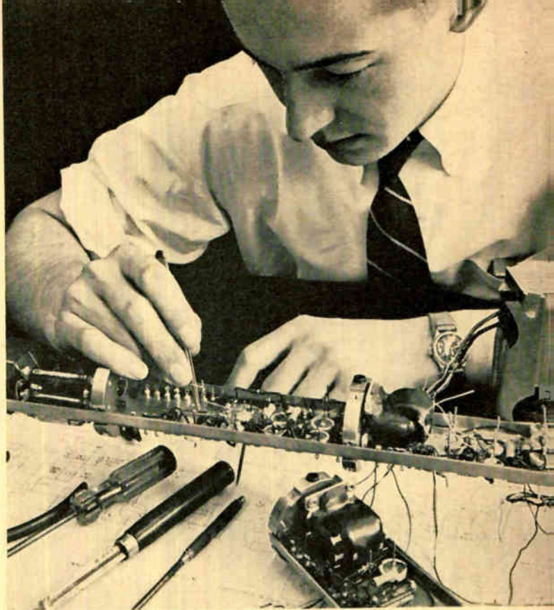
Laboratory technician testing a Schlumberger experimental electronic cartridge for use in logging of bore holes
