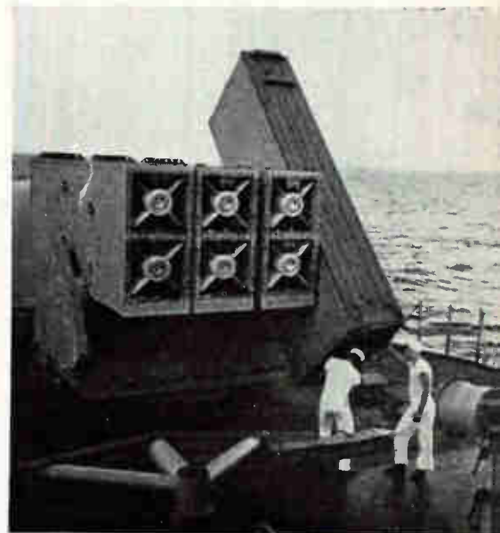
Technicians seal the eight missile cells of electronically controlled launcher before firing
