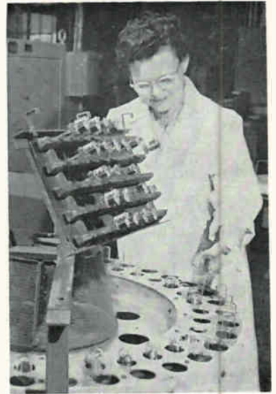
In this pilot production operation at GE, the new tubes are preheated as above on a rotating wheel, then exhausted and sealed
