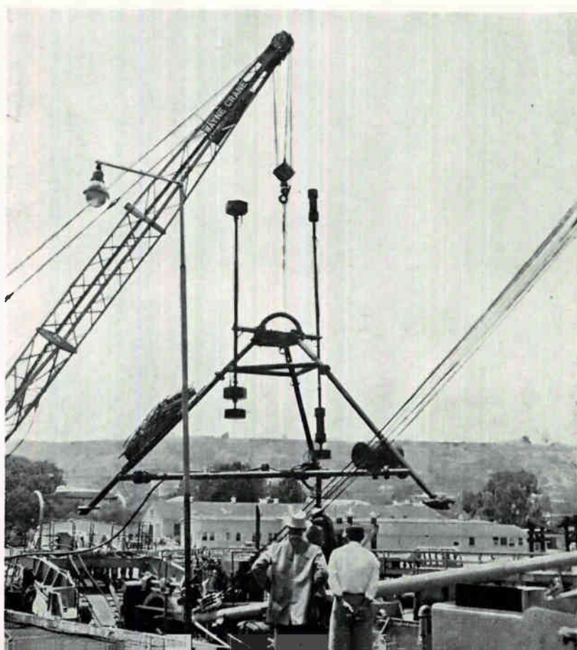
Tripod with hydrophones and other oceanographic equipment is being loaded onto boat. Equipment is used in research on ambient ocean noise, as distinct from man-made or biological noise
