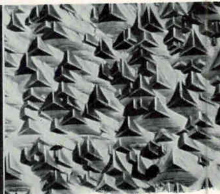
Microsection (left) of vapor-grown germanium-gallium arsenide tunnel diode and typical epitaxial (vapor) growth on the 111 crystallographic plane (right) of a silicon substrate
