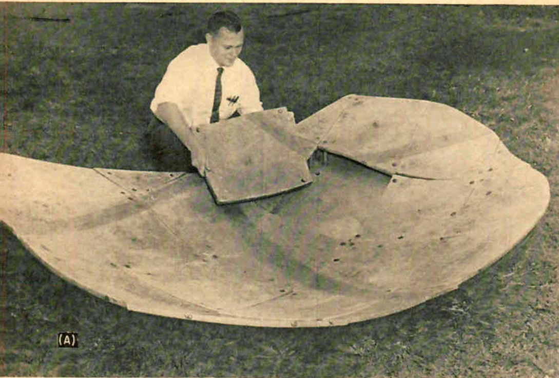
FIG. 5—Scale model of dual parabola antenna reflector that combines both search and height-finding functions (A), multiple focal length lens can be used by two or more radars (B) and steerable mount for large parabolas gives continuous rotation through any point (C)
