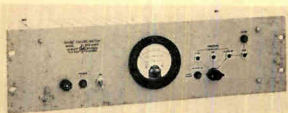
Meter operates from 90 to 500 pps to determine noise figure of radar receiver
