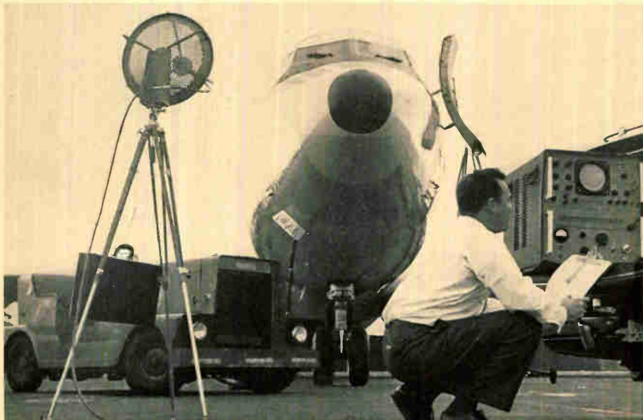
FIG. 1—Navigation systems in long-distance commercial airliners use doppler radar to measure ground speed
