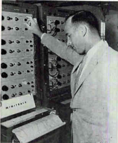
Analog recorder at Florida Minitrack station translates signals 4 times a day from still-busy Vanguard 1
