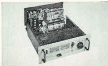
"Flip Top Box" Permits Accessibility For Maintenance
